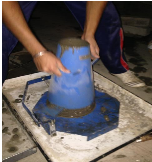
FIGURE 4a – Slump Test
