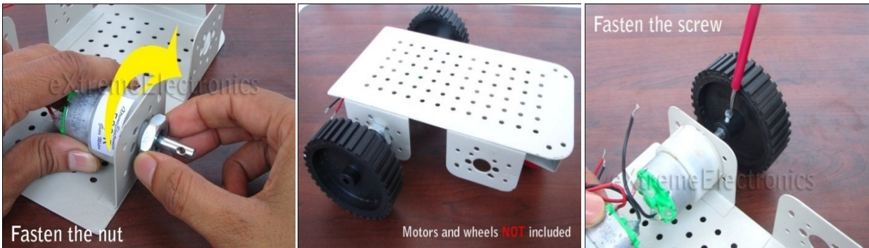
Figure 4.1: Fixing DC Motors and Wheels on the metal chassis
