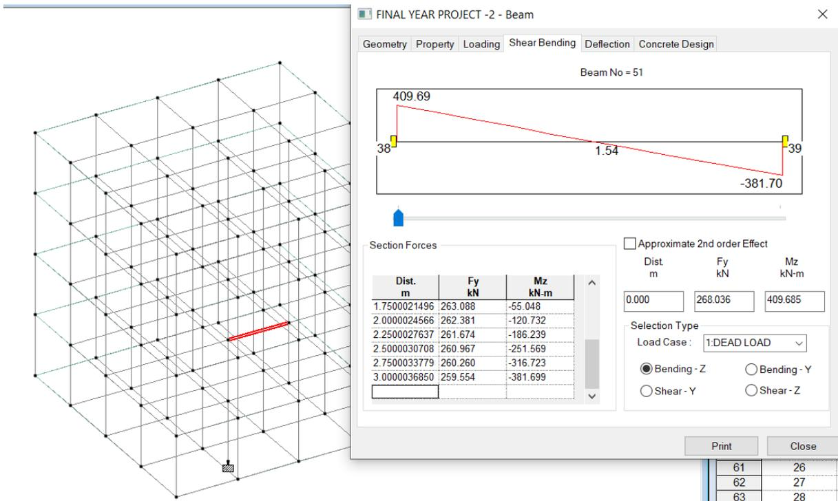
Figure 11.11 Shear bending of beam 51
