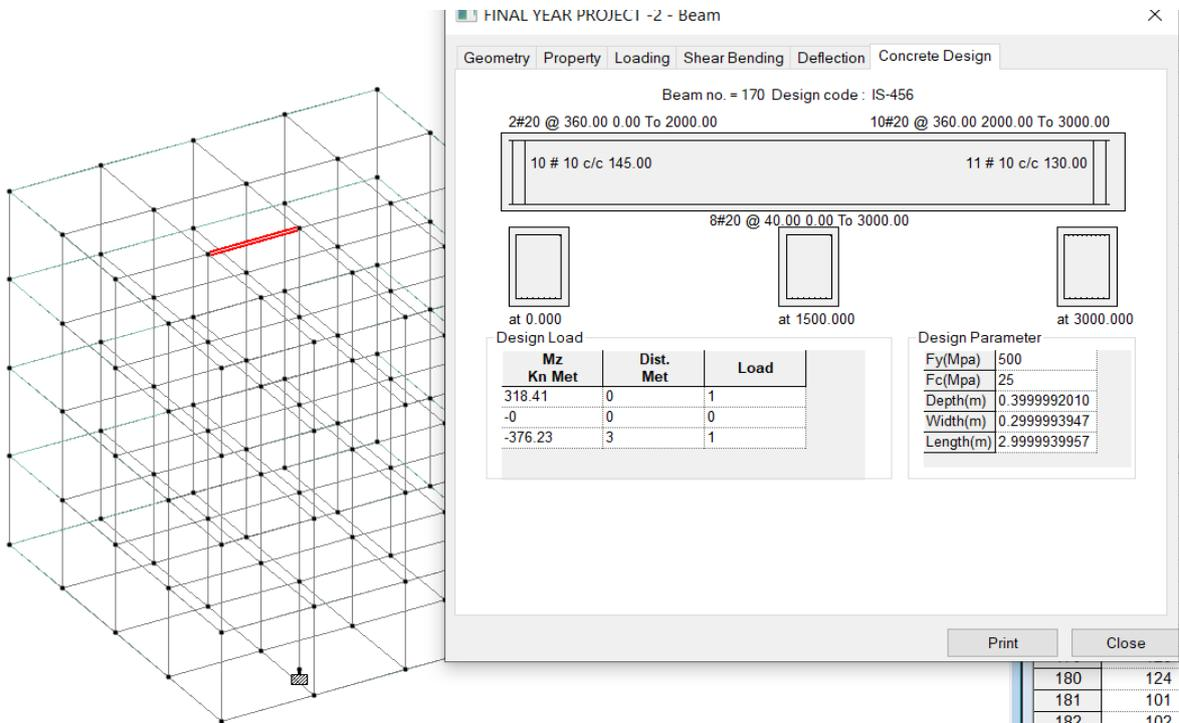
Figure 11.10 Concrete design of beam 170
