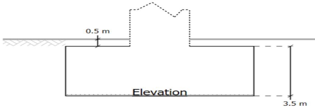
**Figure 8.10** Elevation of isolated footing
