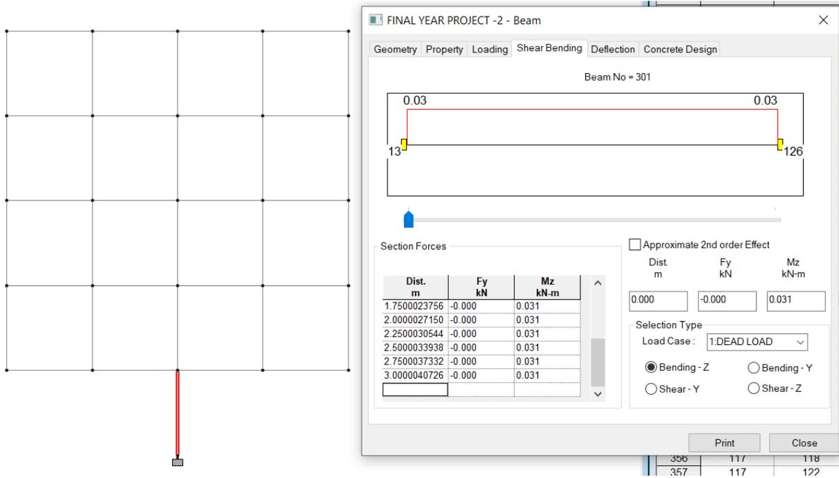
Figure 11.5 Shear bending of beam 301
