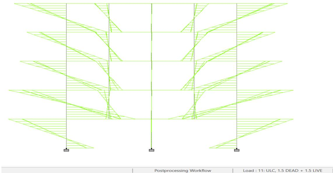
**Figure 9.13** Moment in Y direction for multiple columns structure (VIEW FROM -X)
