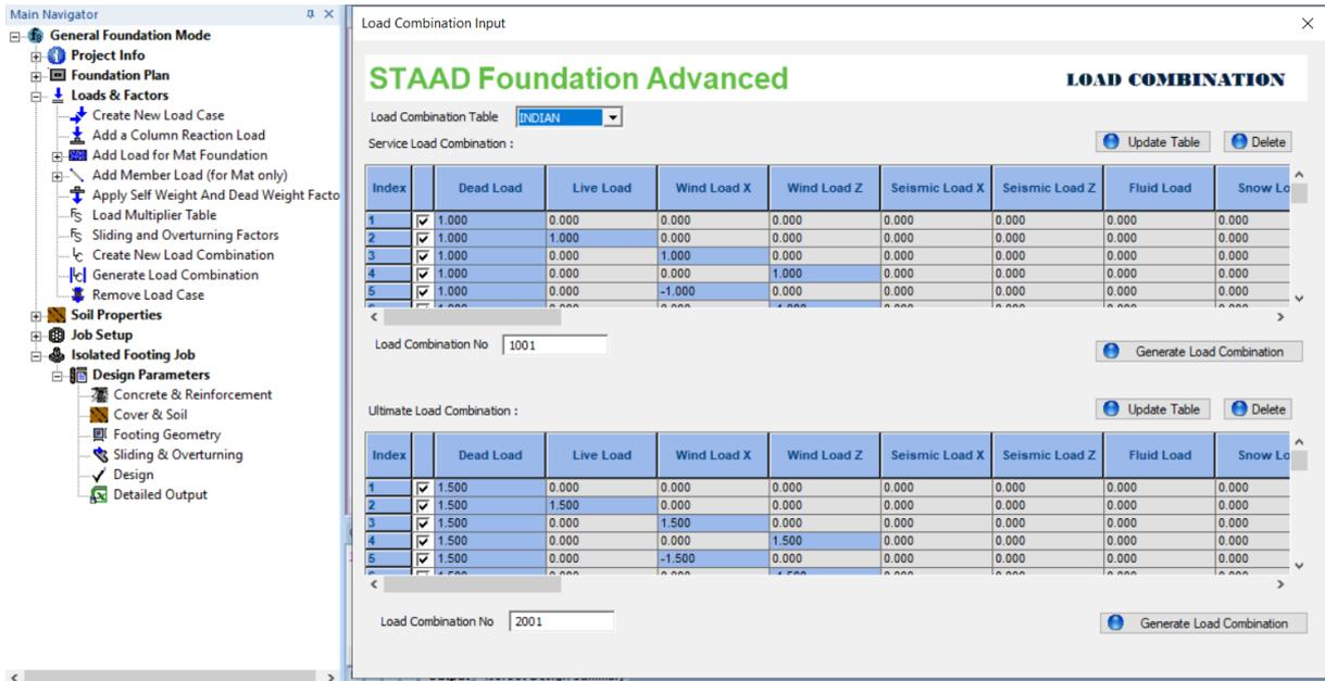
Figure 8.2 Load combination generation table
