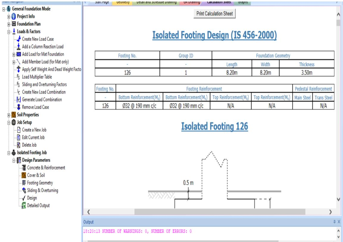
**Figure 8.9** Analysis window showing zero errors with the dimensions of footing
