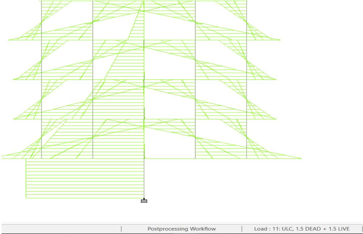
**Figure 9. 12** Moment in Y direction for single column structure(VIEW FROM -X)
