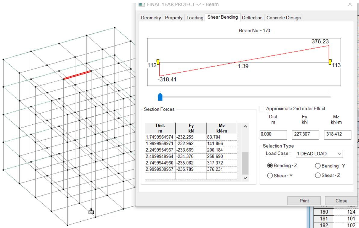
Figure 11.8 Shear bending of beam 170
