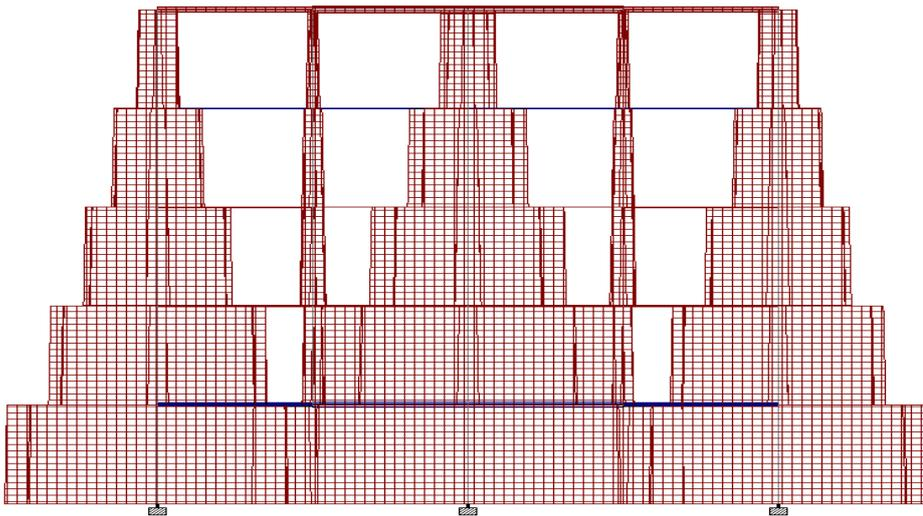
**Figure 9.5** Shear force diagram of  $F_x$  of multiple column building(FRONT VIEW)
