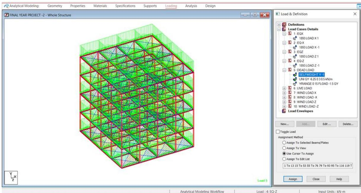
Figure 6.1 Self-weight in -y direction
