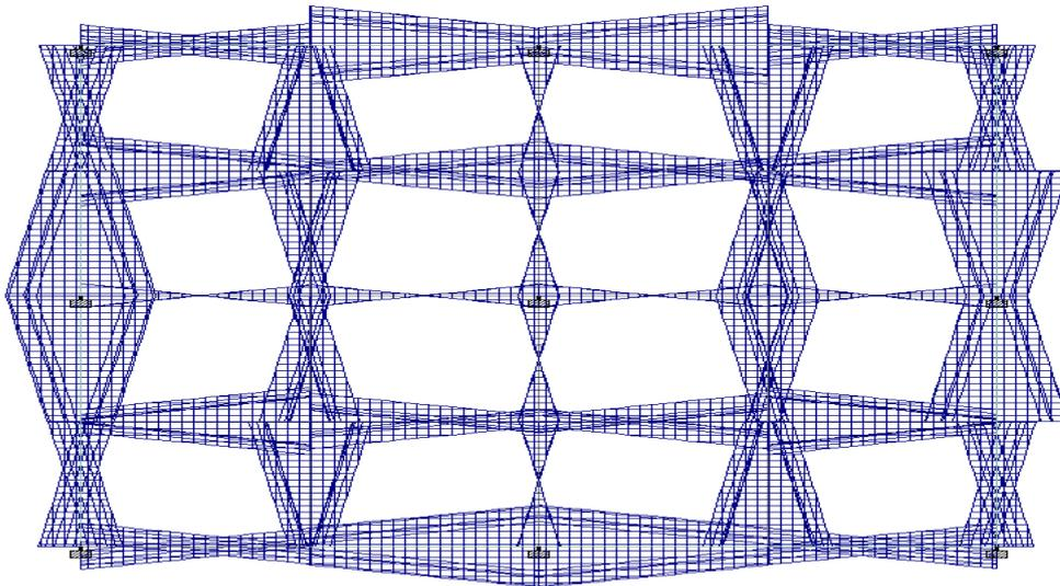
**Figure 9.11** Moment in X direction for multiple columns building(TOP VIEW)
