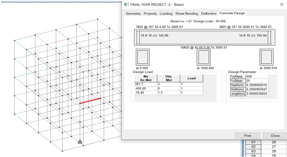
Figure 11.13 Concrete design of beam 51
