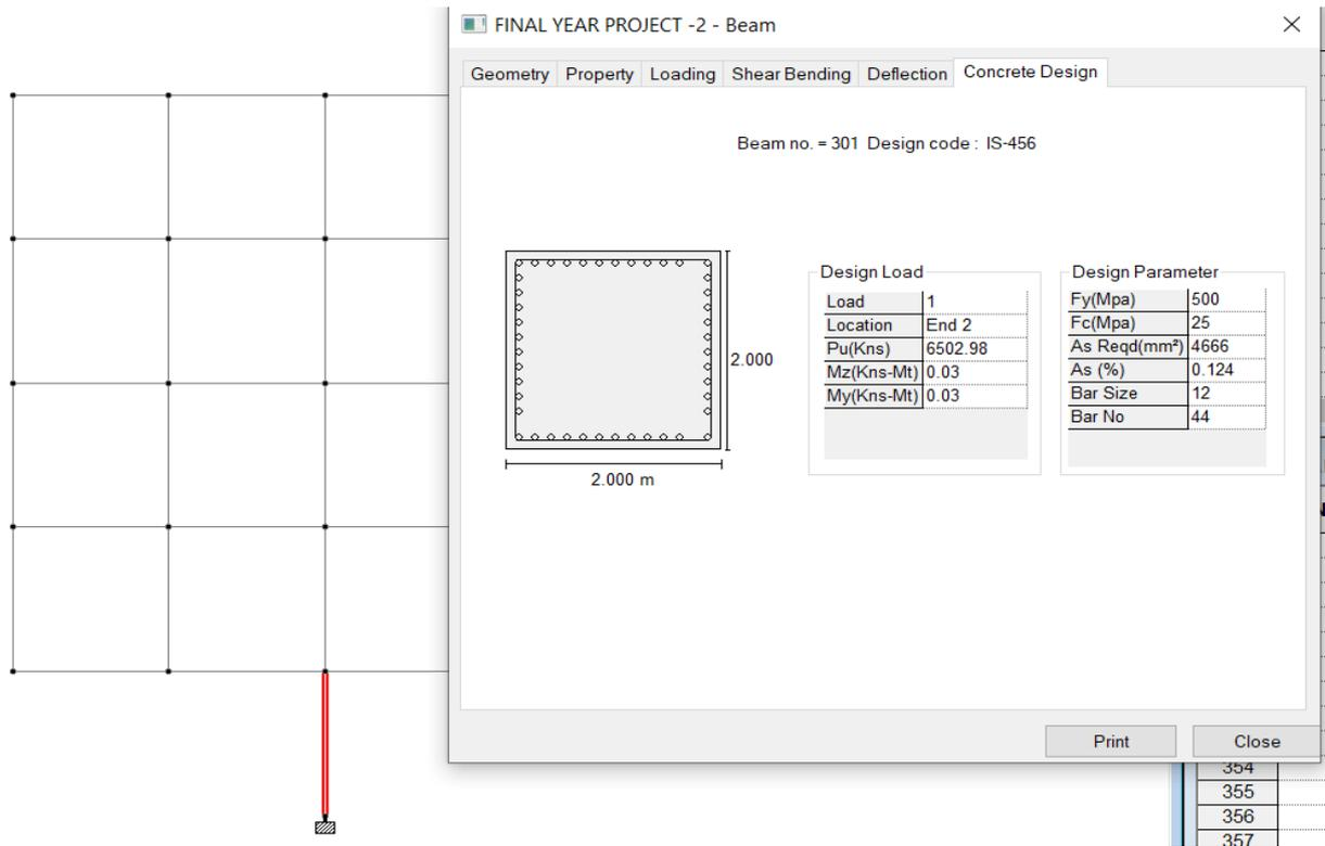
Figure 11.7 Concrete design of beam 301
