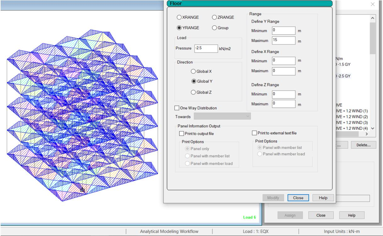
Figure 6.4 Live load of -2.5 k n/m<sup>2</sup> on structure
