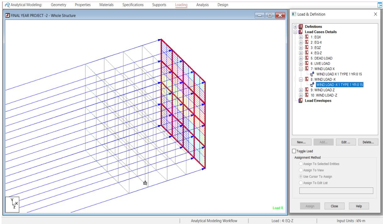
**Figure 6.9** Wind load in -x direction
