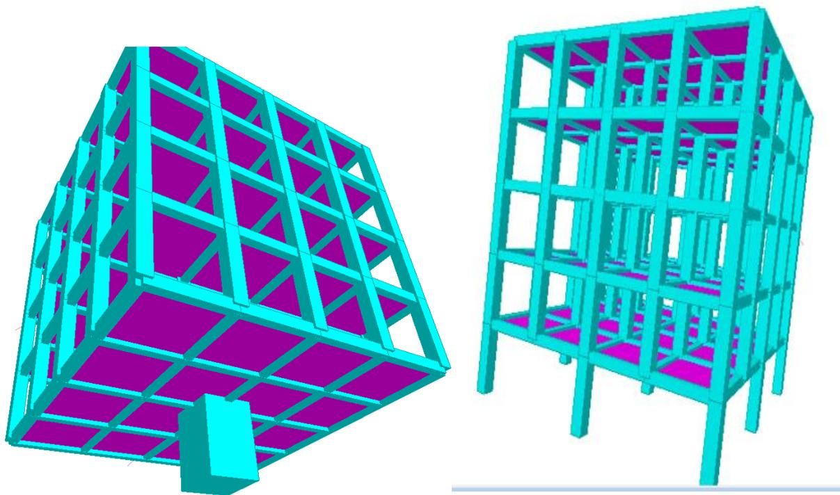
**Figure 9.1** Single column building and multiple columns building used for comparison in project.
