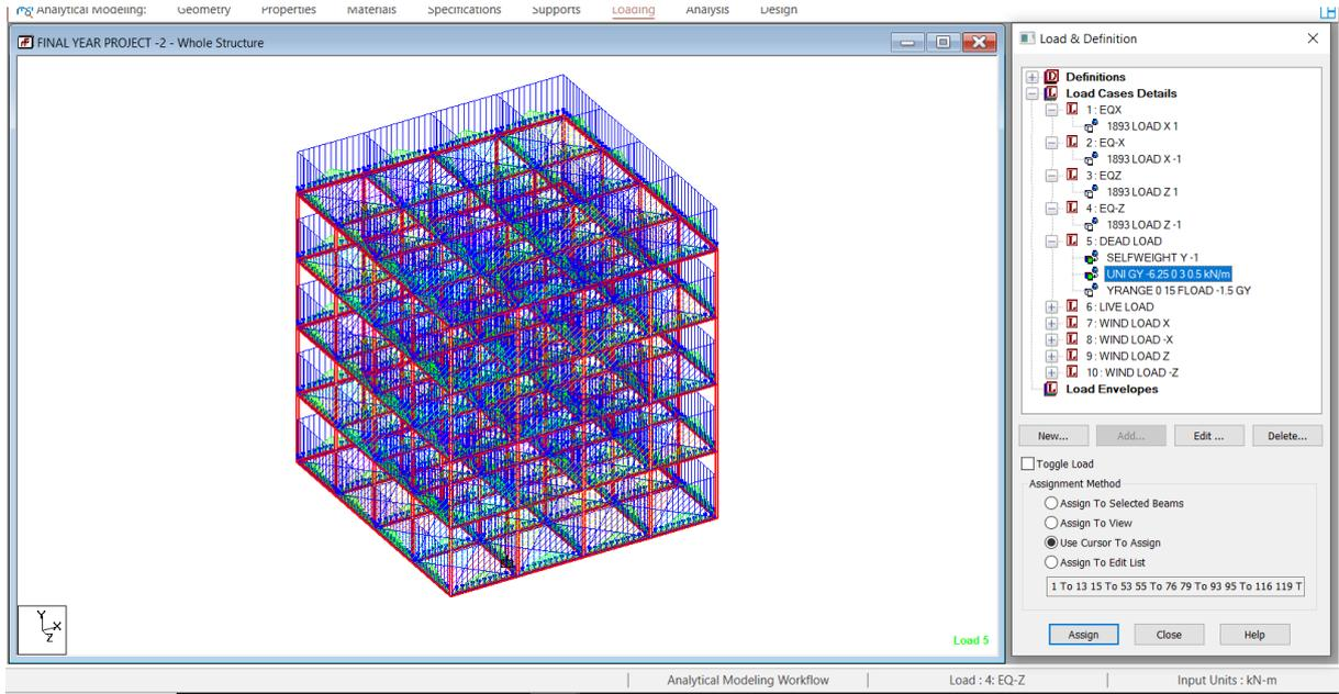
**Figure 6.2** Wall load of  $-6.25 \text{ kN/m}$  on structure.
