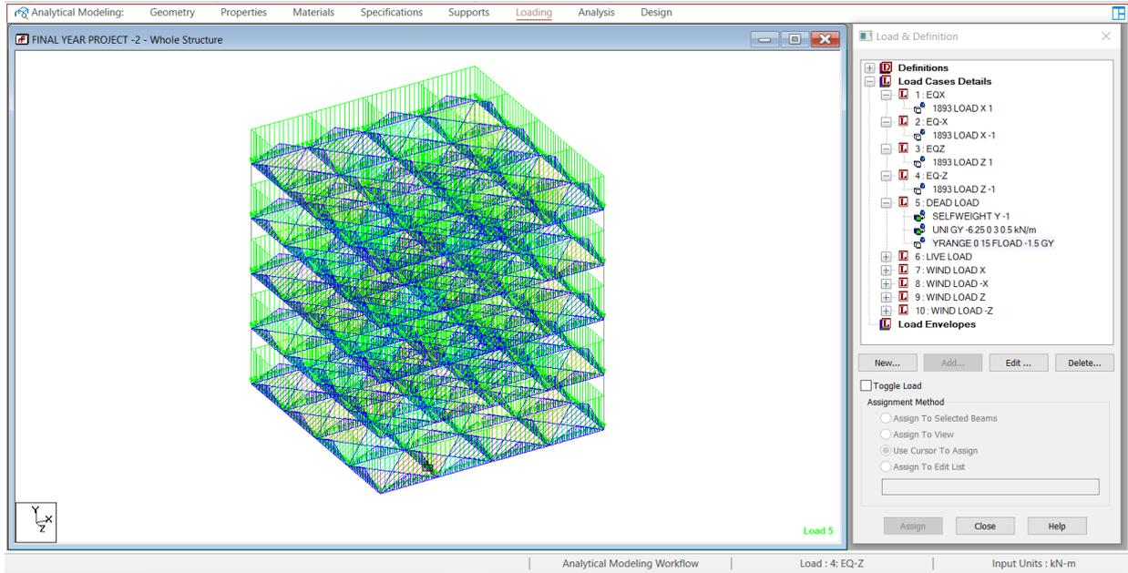
**Figure 6.3** Floor finish of  $-1.5 \text{ k n/m}^2$
