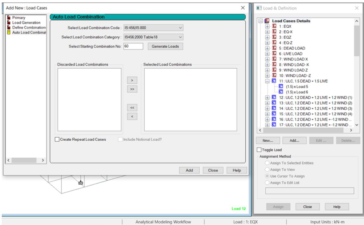
**Figure 6.14** Auto generating load combinations as per is 456.
