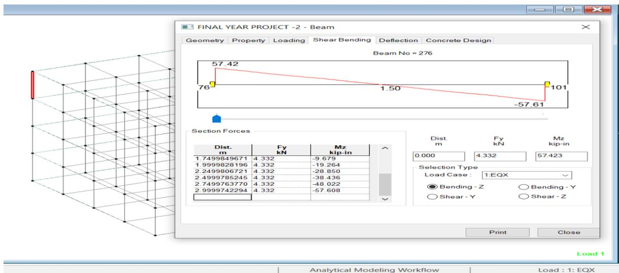
Figure 11.16 Beam 276 shear bending
