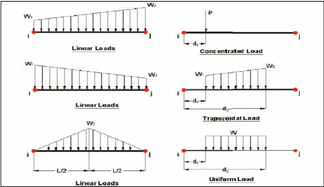
**Figure 4.2 Member load configuration**
