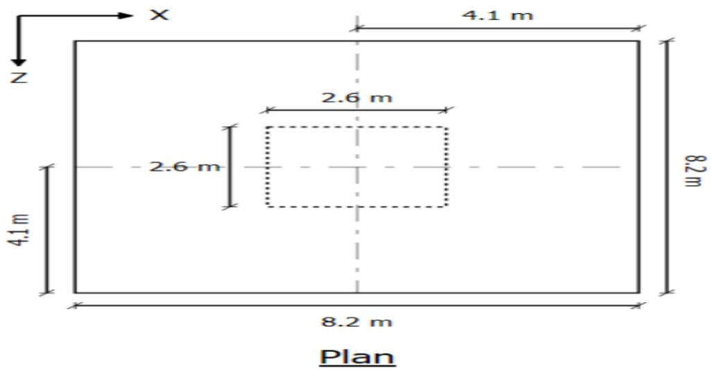
**Figure 8.11** Plan of isolated footing
