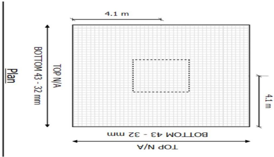
**Figure 8.12** Reinforcement summary of foundation
