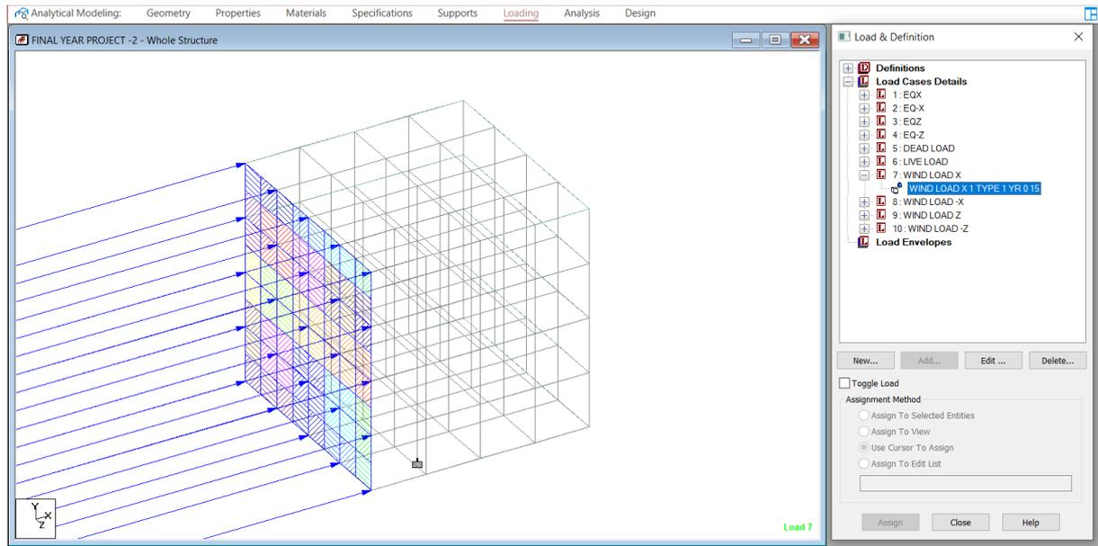
**Figure 6.8** Wind load in +x direction
