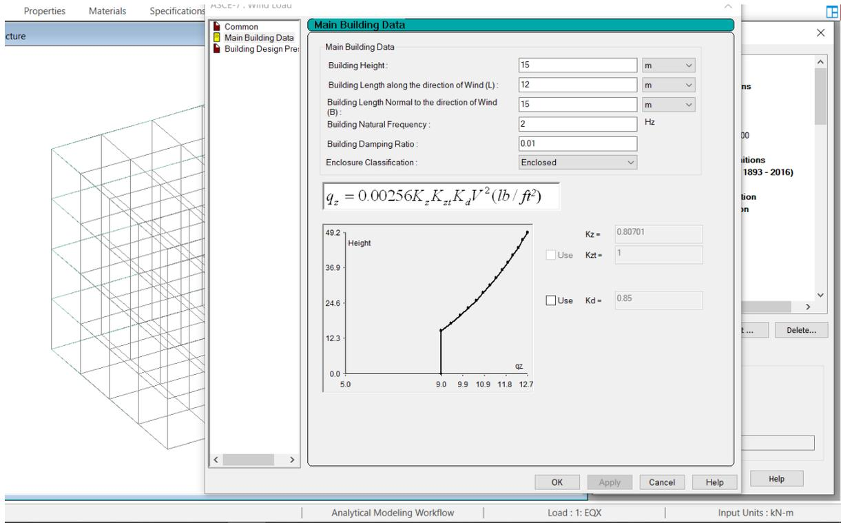
**Figure 6.7** Main building data for wind load
