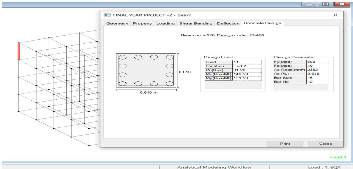
Figure 11.18 Concrete design of beam 276
