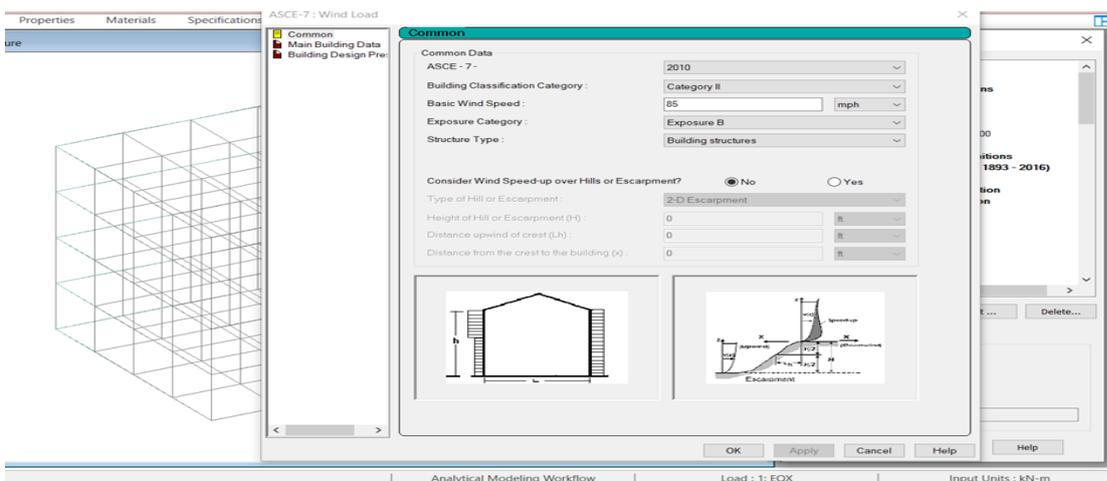
**Figure 6.6** Input parameters for wind load
