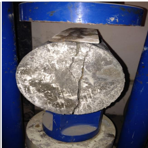
(a) Plain concrete failure pattern
