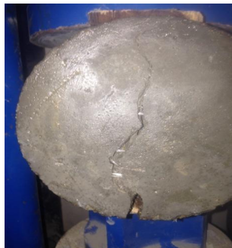
(b) FRC with 0.1% fiber failure pattern
