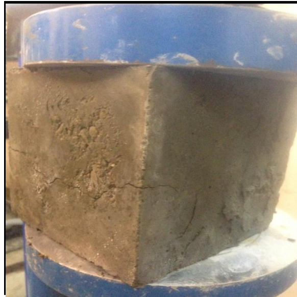
(b) Cracks after failure
