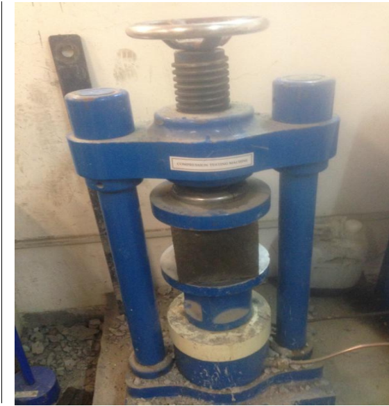
(a) Placing specimen on CTM
