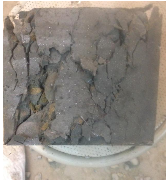
(b) Cube specimen with 0.1% fiber content
