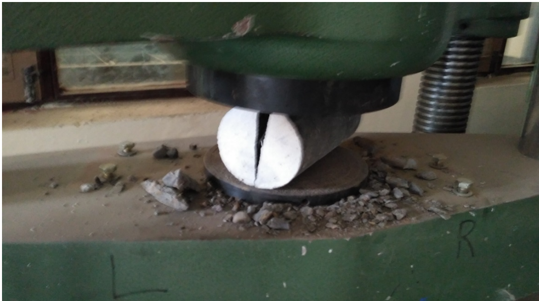
Fig. 4.9 Brittle failure of cylinder without fibre
