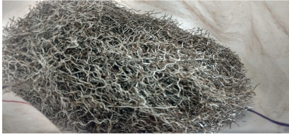
Fig. 3.2 Steel fibre used in project
