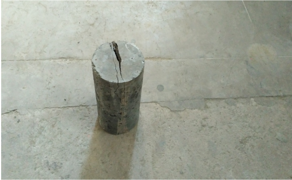
Fig. 4.13 Failure of cylinder with fibre
