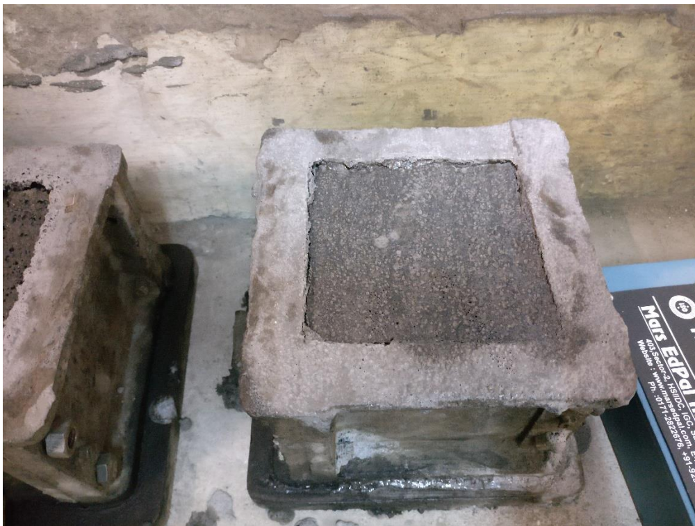
Figure A.3: Specimen after 24 hrs prepared for demolding
