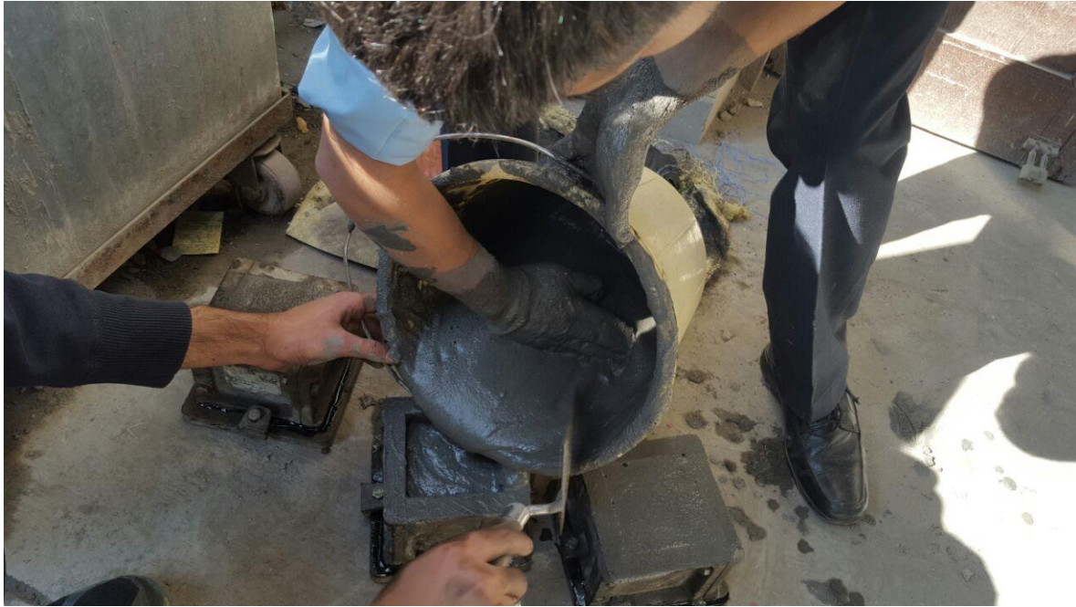
Figure A.2: Casting of Specimen
