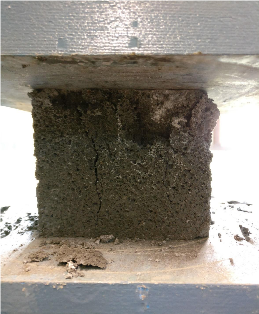
Figure A.1: Compressive Test being performed on specimen
