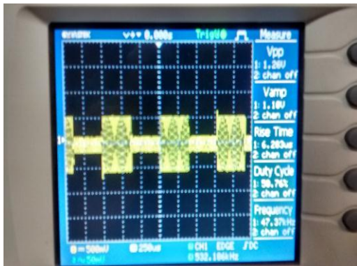
Figure 4.4-5: modulated wave received at receiver in 50cm range
