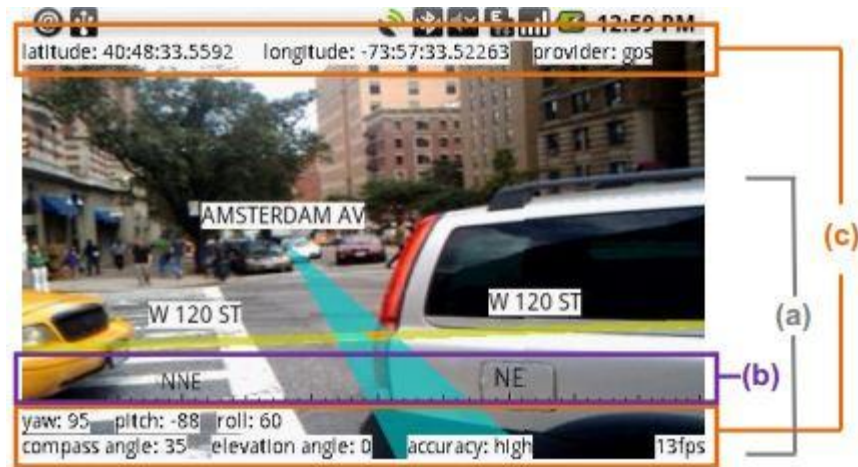
Figure 6: AR street view 3D components. (a) Street objects are registered with the real world and annotated with labels. (b) Compass reticle shows heading. (c) Information display shows the quantitative values of GPS, orientation, and other sensor observations.
