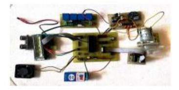
As shown in the above, node2 consists of motion detector, temperature sensor, humidity senor, cooling fan, water pump, etc. connected to the microcontroller board. The sensors give input to the controller and according to that microcontroller controls the devices in auto mode and also sends the value of sensors to R-Pi and R-Pi forwards it to user's smart device using internet. Test results shows that when temperature level increases above preset threshold
