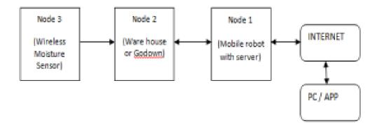
This paper is composed of 4 parts-Node1, Node2, Node3 and PC for controlling the required system. Each node is combined with several sensors and policy. They are organized systematically in one main server through wireless communication modules.
