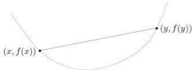
Fig.2.1 Graph of a convex function. The chord (i.e., line segment) between any two points on the graph lies above the graph.
