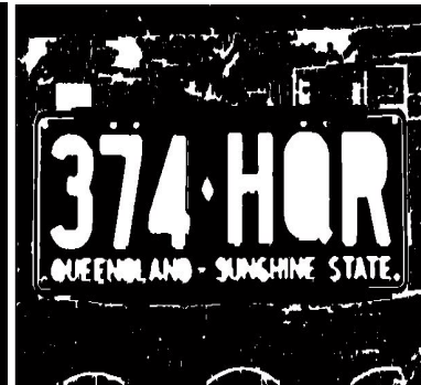
Fig2.18: Elimination of possible horizontal lines, via erosion function using line structuring element, from the output image of regiongrow that could possibly be the horizontal edges(borders) of the license plate.
