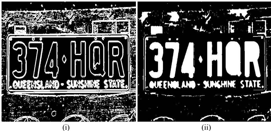
Fig2.19: Character Filling, Character Thinning and Erosion is performed
