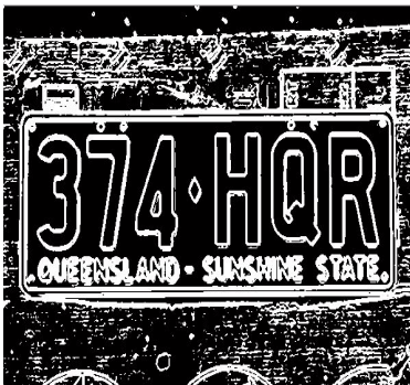
Fig2.18: Elimination of possible horizontal lines, via erosion function using line structuring element, from the output image of regiongrow that could possibly be the horizontal edges(borders) of the license plate.
