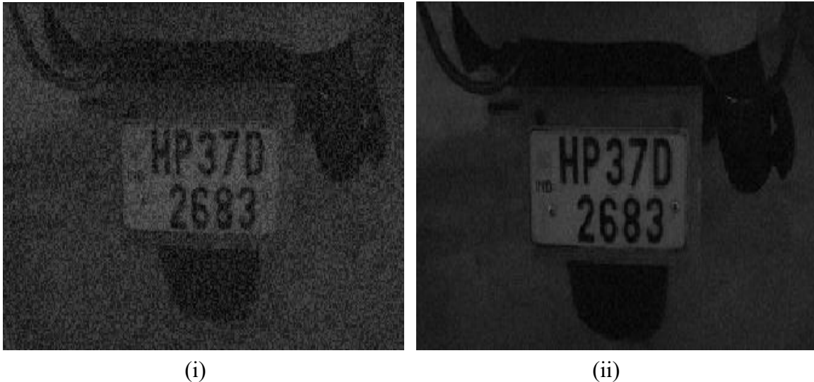
Fig2.10: Effect of Median Filter on Salt and Pepper Noise
