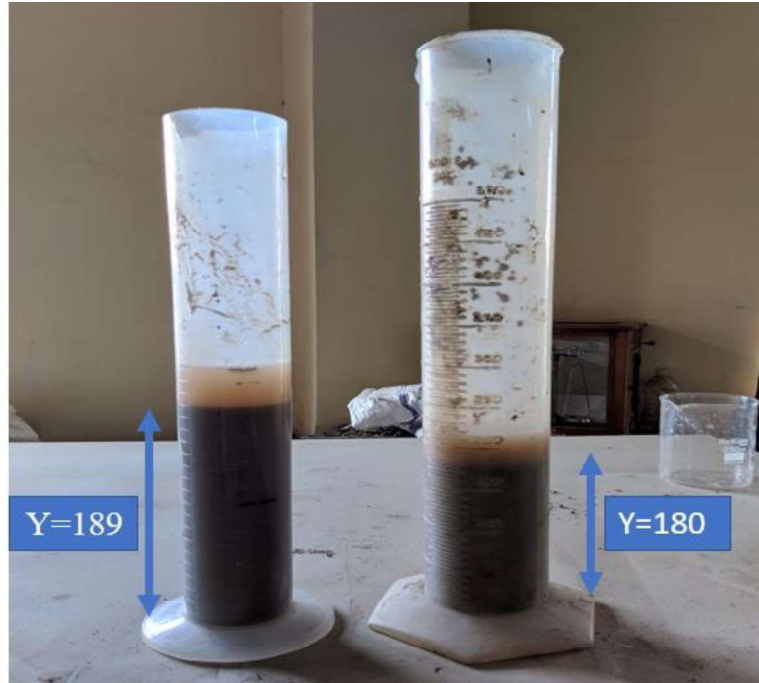
Fig.3.5: Measuring cylinder of silt content experiment
