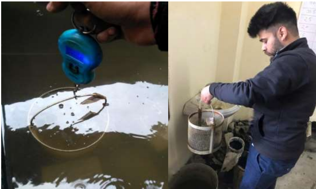
Figure 3.8- (a) Weighing aggregates in basket in water (b) Weighing of aggregates in basket in air
