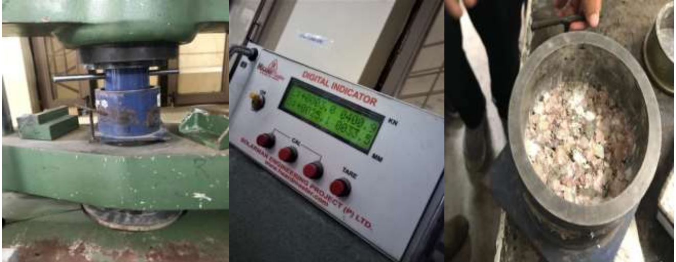
Figure 3.3- (a) Sample under Universal testing machine (b) Readings of UTM (c) Sample after testing
