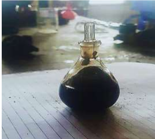
Figure 3.12 Specific Gravity Bottle
