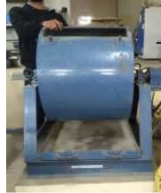
Figure 3.4 Los Angeles Abrasion apparatus
