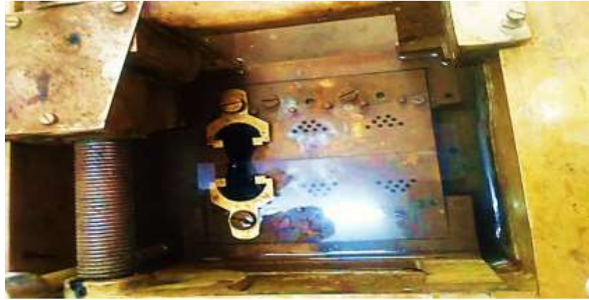
Figure 3.11 Ductility Test Apparatus
