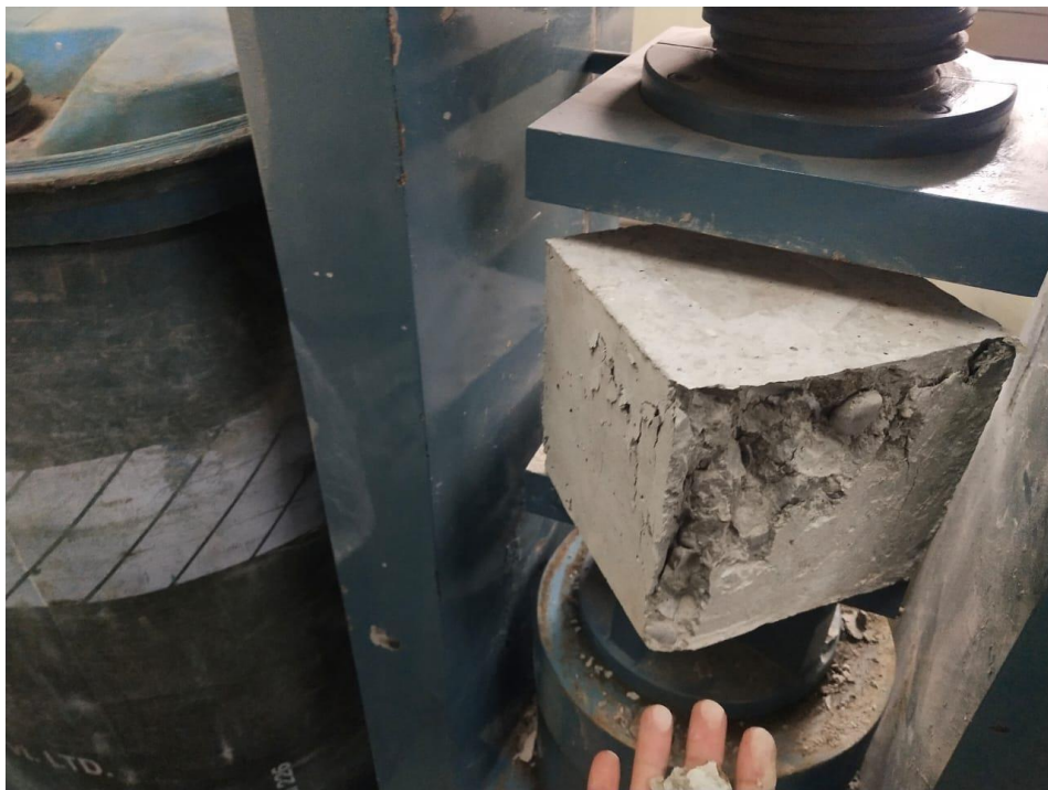
Figure 4.3 Cube failed while testing under CTM
