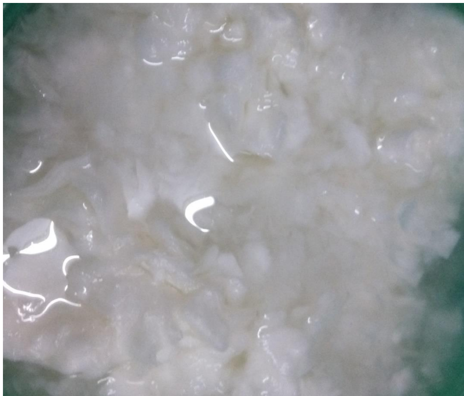
Figure 3.2 Cellulose fibers in Slurry form
