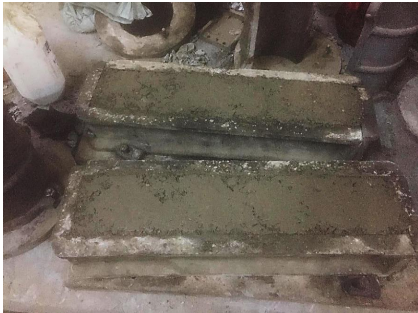
Figure 3.7 Beam of concrete to test flexural strength
