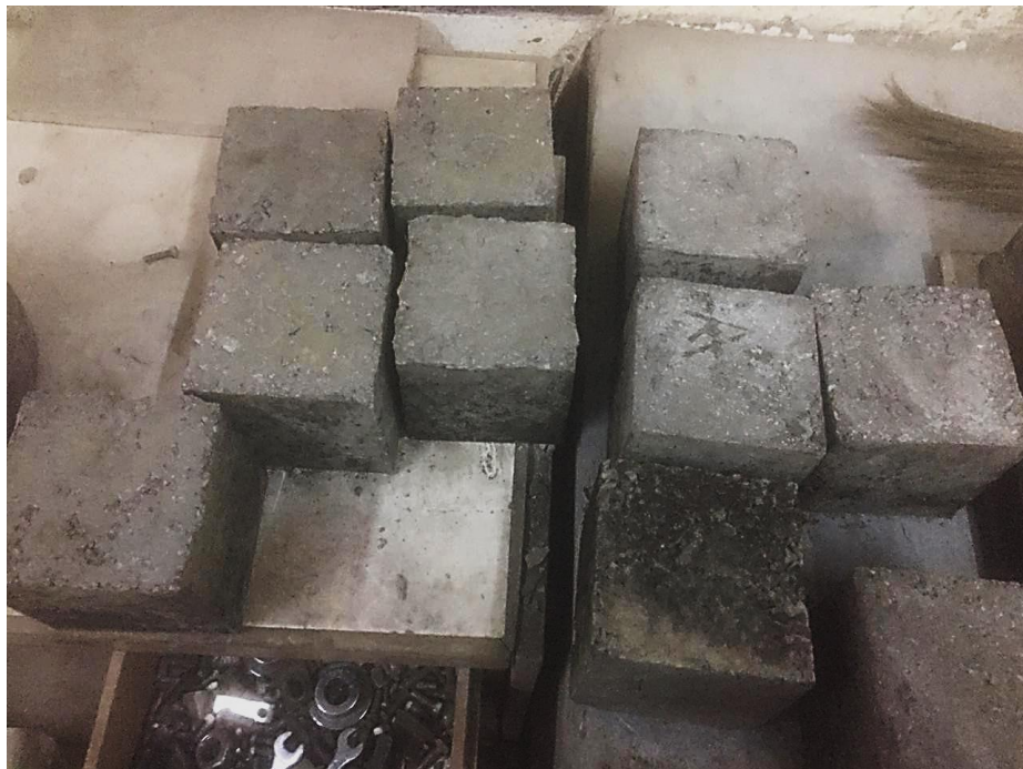
Figure 3.9 Concrete cubes casted with 0.5% of cellulose fiber
