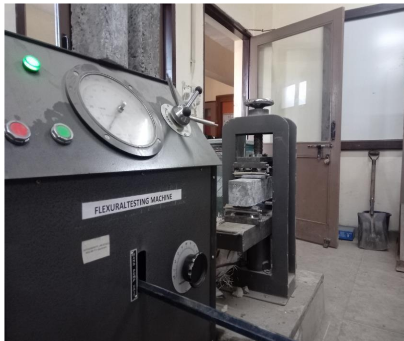
Figure 3.12 Machines to test Flexural strength
