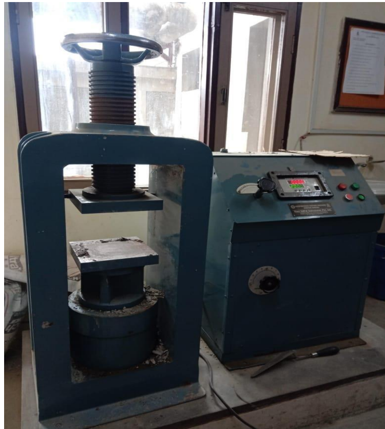
Figure 3.11 CTM with 2000KN capacity
