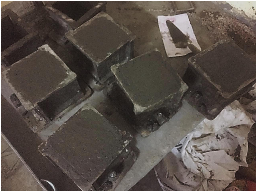
Figure 3.8 Cube of Concrete to test compressive strength
