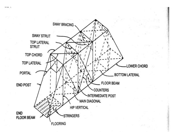
Figure 1.2 Components of a Truss Bridge<sup>[2]</sup> Source- Victor(2012)
