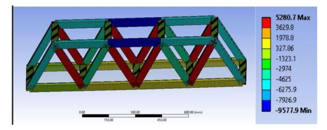
Figure 4.3 Areas of Axial Force according to the values
