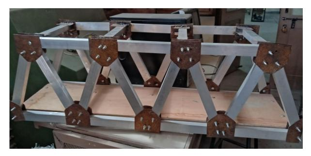
Figure 3.18 Image of Model made using hollow sections.
