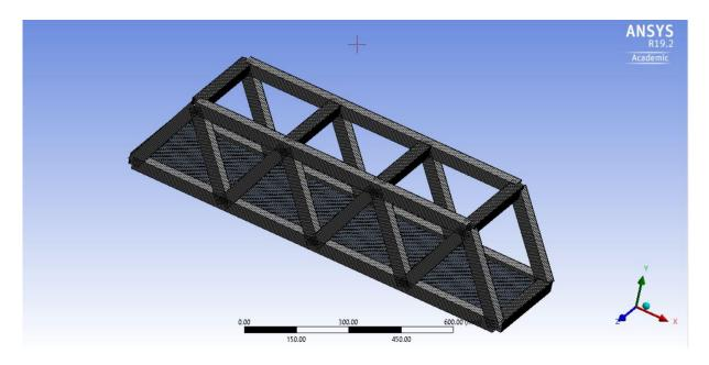
Figure 3.15 Meshed Geometry of the bridge.
