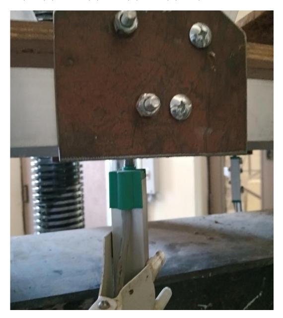
Figure 3.20 LVDT attached at a node.
