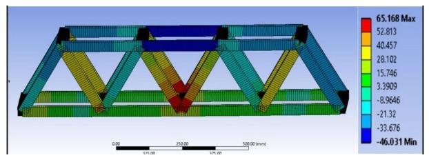
Figure 4.6 Areas of Maximum Combined Stress according to the values
