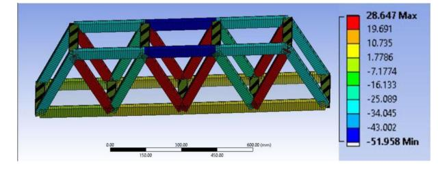
Figure 4.4 Areas of Direct Stress according to the values
