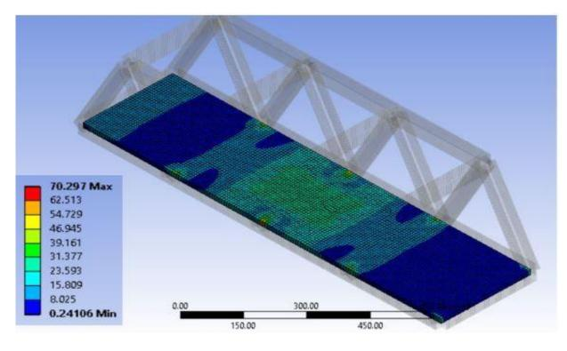
Figure 4.2 Areas of Equivalent Stress according to the values
