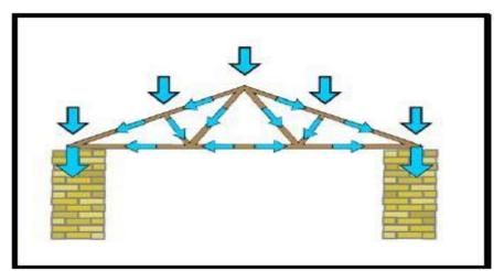
**Figure 3.1** Distribution of load over a truss bridge<sup>[13]</sup> Source- Jasim(2016)
