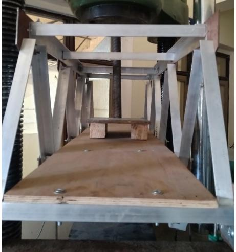
Figure 3.23 Image of Load Imprint provided on the deck of bridge prototype
