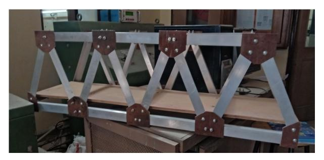
Figure 3.17 Image of Model made using angle sections.
