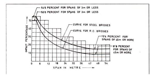
Figure 3.6 Impact percentage Curve<sup>[14]</sup> IRC-6 (2014)
