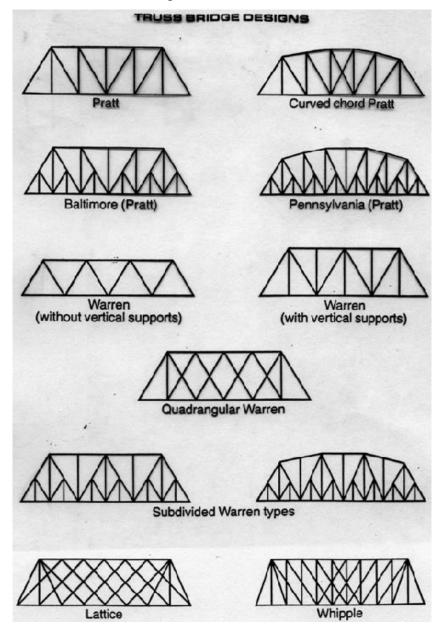
Figure 1.1 Typical Bridge Trusses<sup>[2]</sup> Source- Victor(2012)
