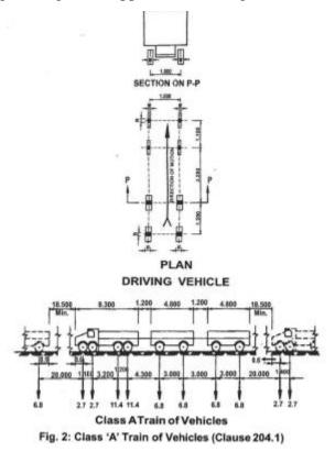
Figure 3.4 Class A loading Imprint Details<sup>[14]</sup> IRC-6 (2014)
