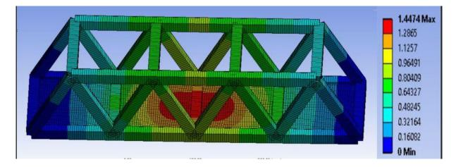
Figure 4.1 Areas of Total Deformation according to the values.
