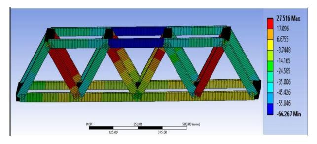
Figure 4.5 Areas of Minimum Combined Stress according to the values
