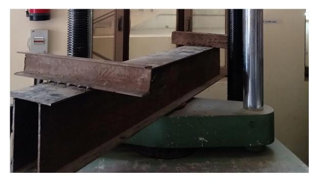
Figure 3.24 support system used in bridge Testing
