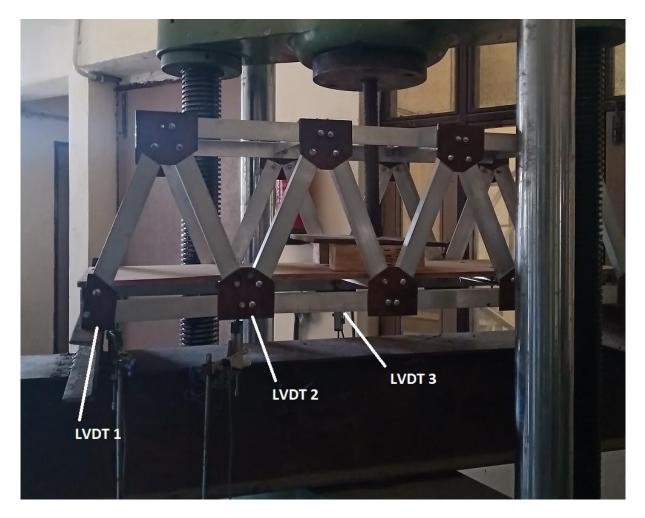
Figure 4.7 Locations of LVDTs
