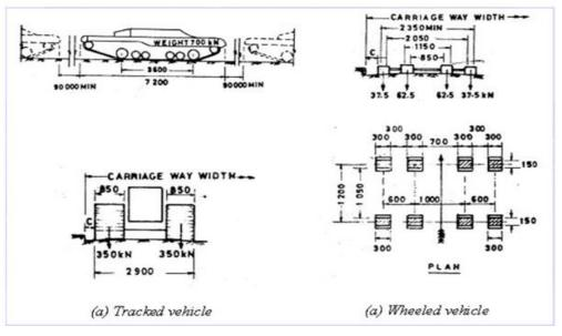
Figure 3.3 Class AA loading Imprint Details<sup>[14]</sup> IRC-6 (2014)
