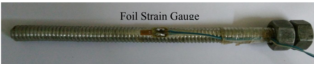
Fig. 3.2.2.(a) Screw nail Fitted with Foil Strain Gauge
