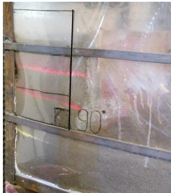
Fig 4.3.5(b) Slope after failure
