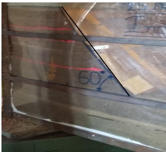
Fig 4.4.3(a) Slope before failure
