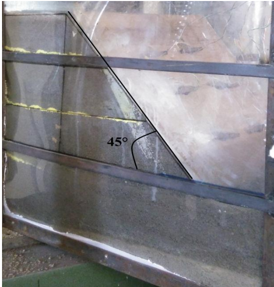
Fig 4.4.1(a) Slope before failure
