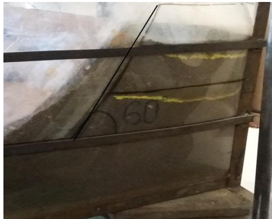
Fig 4.4.4(b) Slope after failure
