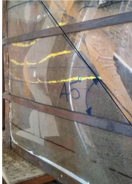
Fig 4.3.2(b) Slope after failure
