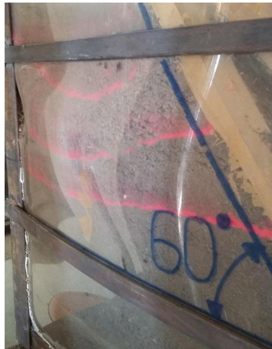
Fig 4.3.4(b) Slope after failure
