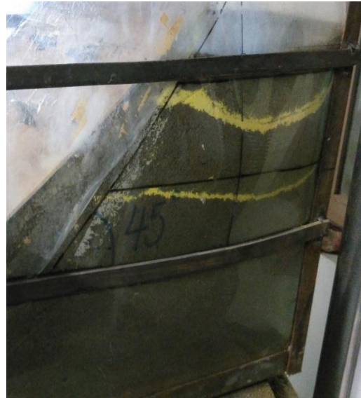
Fig 4.4.1(b) Slope after failure
