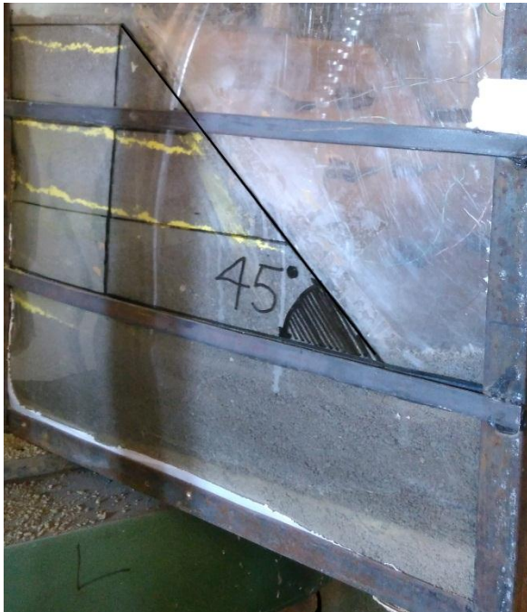
Fig 4.4.2(a) Slope before failure
