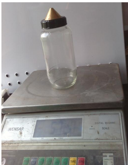
Fig 3.3.2 (a) M_1 Mass of empty pycnometer bottle
