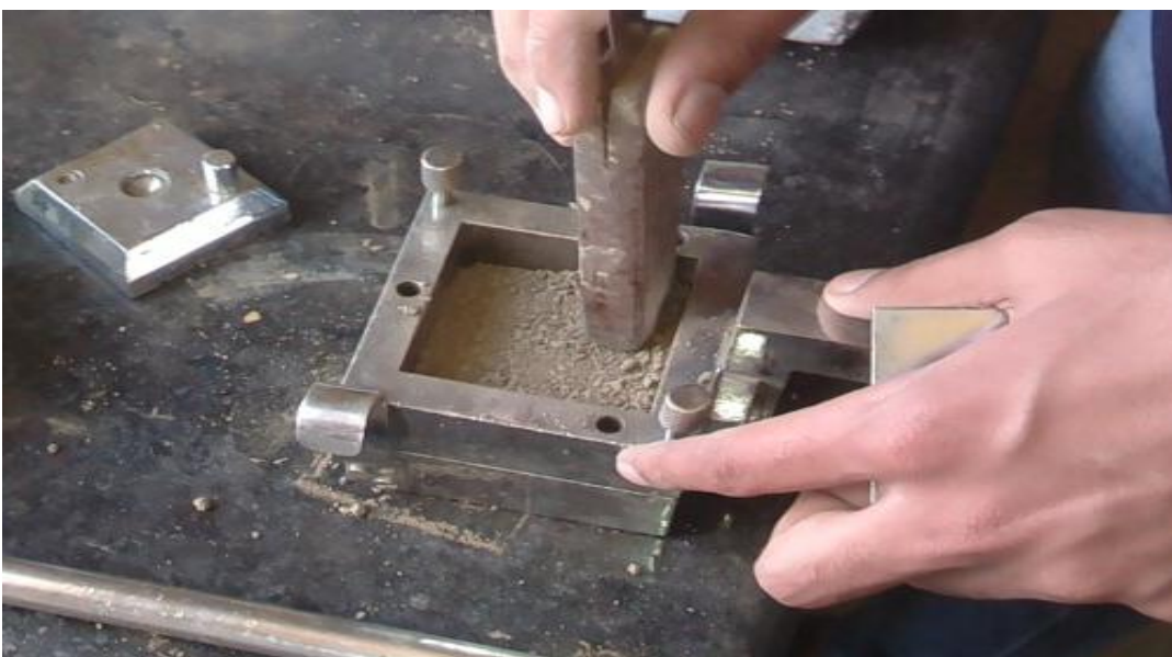
Fig. 3.3.3 (b) Soil Sample Preparation
