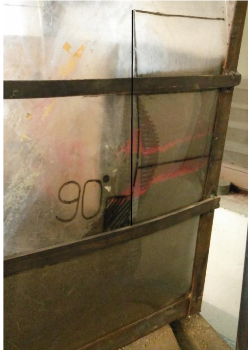
Fig 4.3.6(b) Slope after failure
