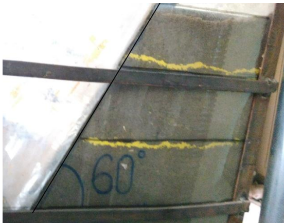
Fig 4.4.4(a) Slope before failure
