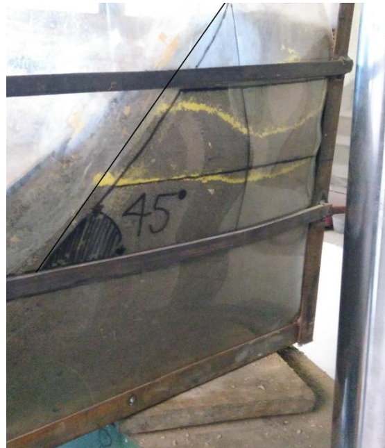
Fig 4.4.2(b) Slope after failure
