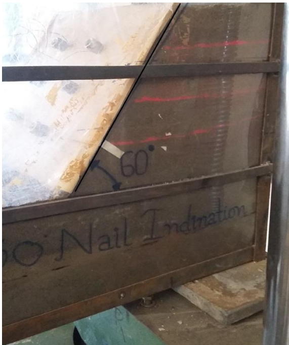
Fig 4.3.4(a) Slope before failure
