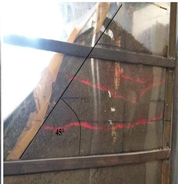
Fig 4.3.1(b) Slope after failure
