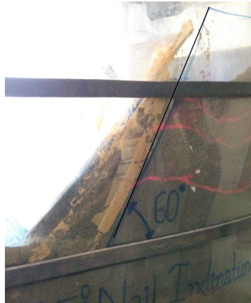
Fig 4.3.3(b) Slope after failure
