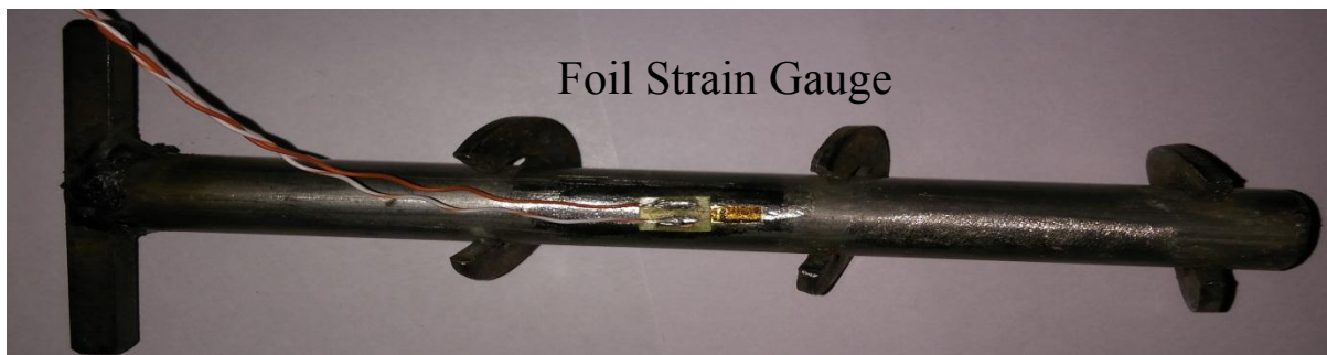
Fig. 3.2.2.(b) Helical nail Fitted with Foil Strain Gauge
