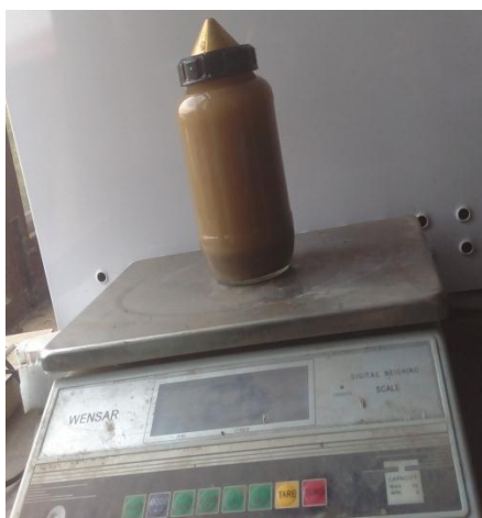
Fig 3.3.2 (b) M_2 Mass of pycnometer with soil and water
