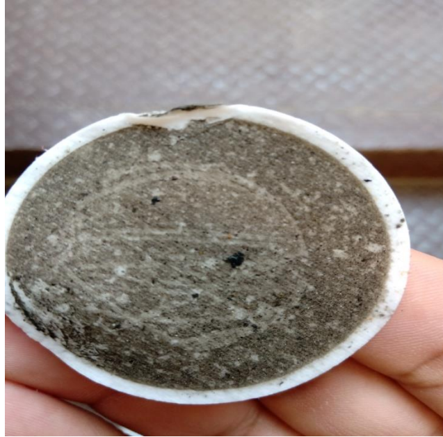
Fig 3.6 Filtration of solid particles from waste water
