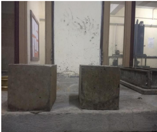
Fig 3.16 Cubes before the curing process
