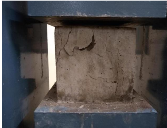
Fig 4.3 Load applied on cubes
