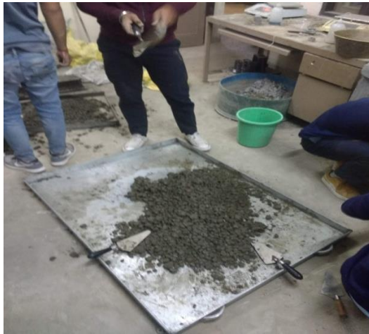
Fig 3.15 Hand mixing of concrete
