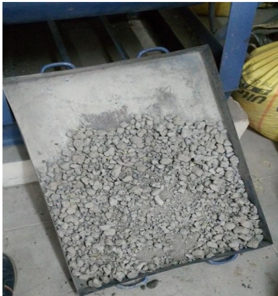
Figure 4.15 RA before water-wash and grading
