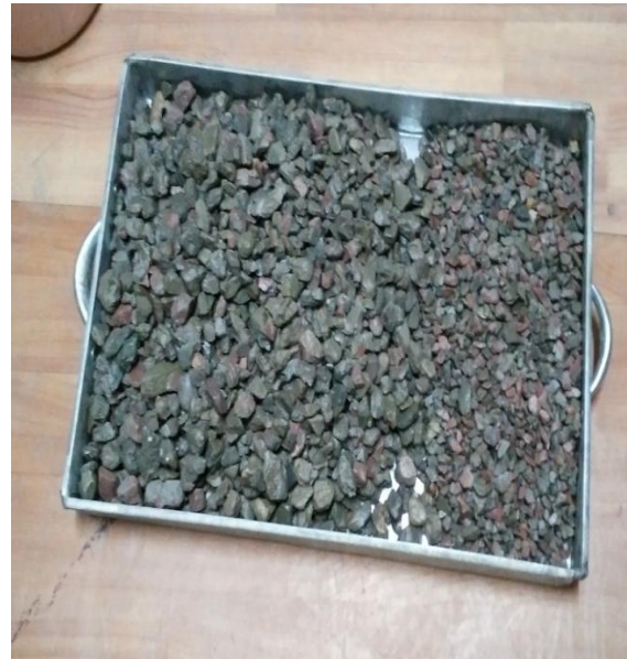
Figure 4.16 Processed RA after water wash
