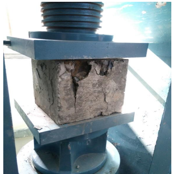
Figure 4.12 Broken element on CTM
