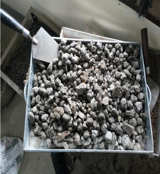
Figure 4.17 Un-processed recycled aggregate
