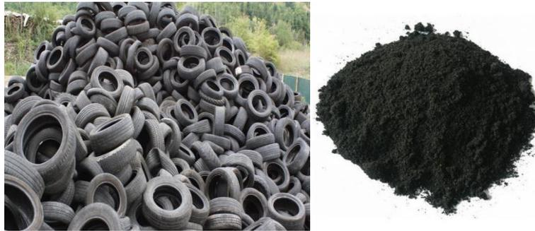
**Figure 1.4** Scrap tyres and crumb rubber
