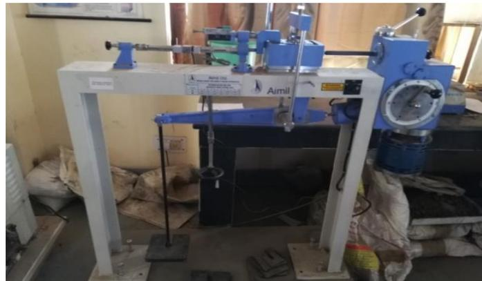
Figure 3.11 Direct shear test apparatus
