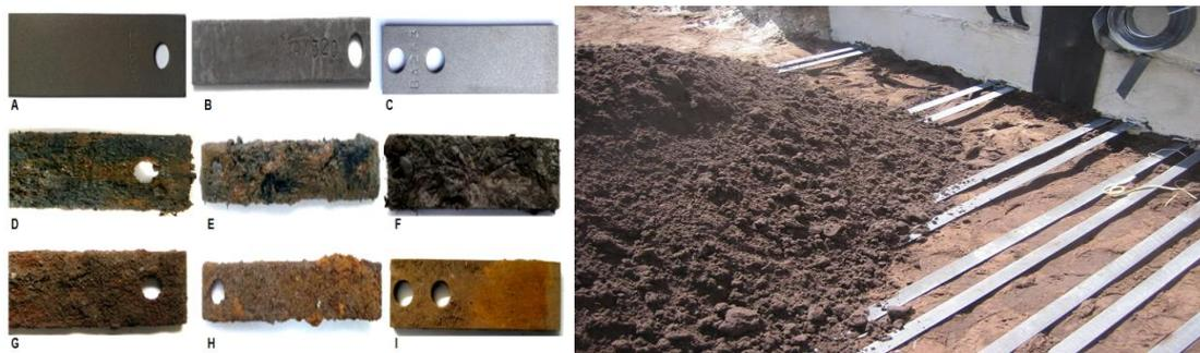
**Figure 1.2** Corrosion in steel reinforcement
