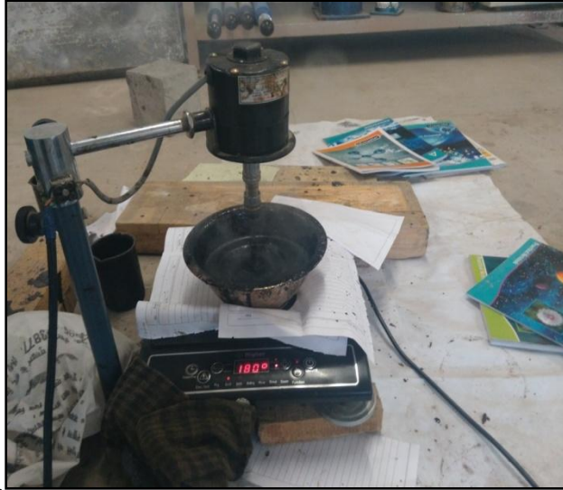
Figure 3.10: Mechanical Mixing of CRMB rubber with bitumen
