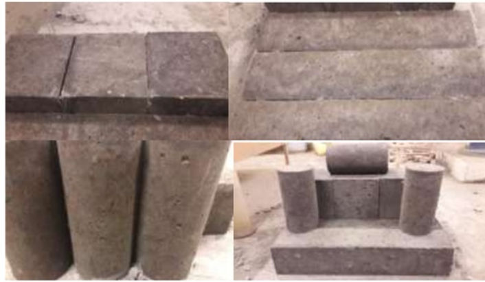
Figure 3.8 Cubes, Beams and Cylinder specimens used in testing
