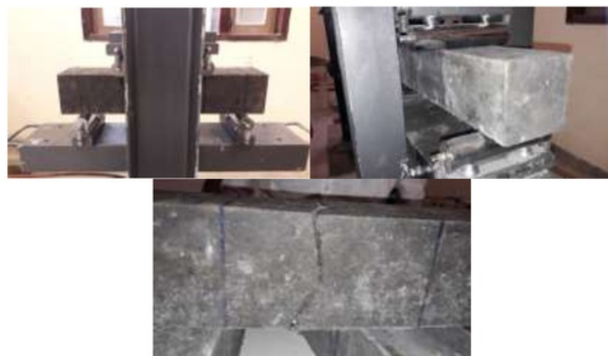
Fig.3.8.3 testing for flexural strength of beams and failed specimen
