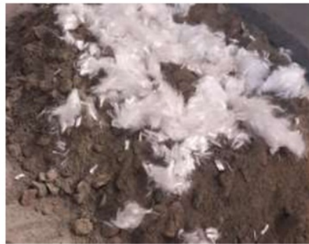
Fig.1.10. Polypropylene fibres before mixing with the concrete materials
