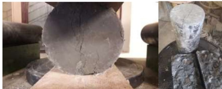
Fig. 3.8.2 testing cylinders for split tensile strength and failed samples
