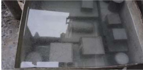
Figure 3.7 Curing of Specimens in Curing Tank
