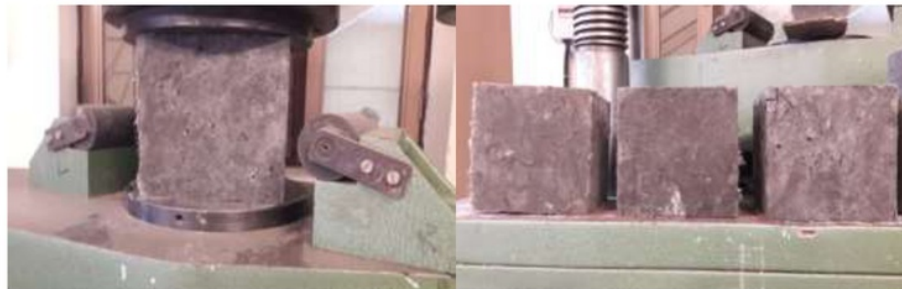
Fig. 3.8.1 compressive testing of cubes in UTM
