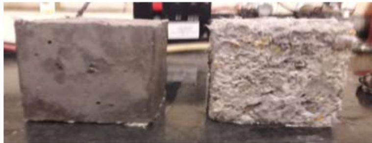
Figure 4.4 Cube after the Alkali and Acid respectively
