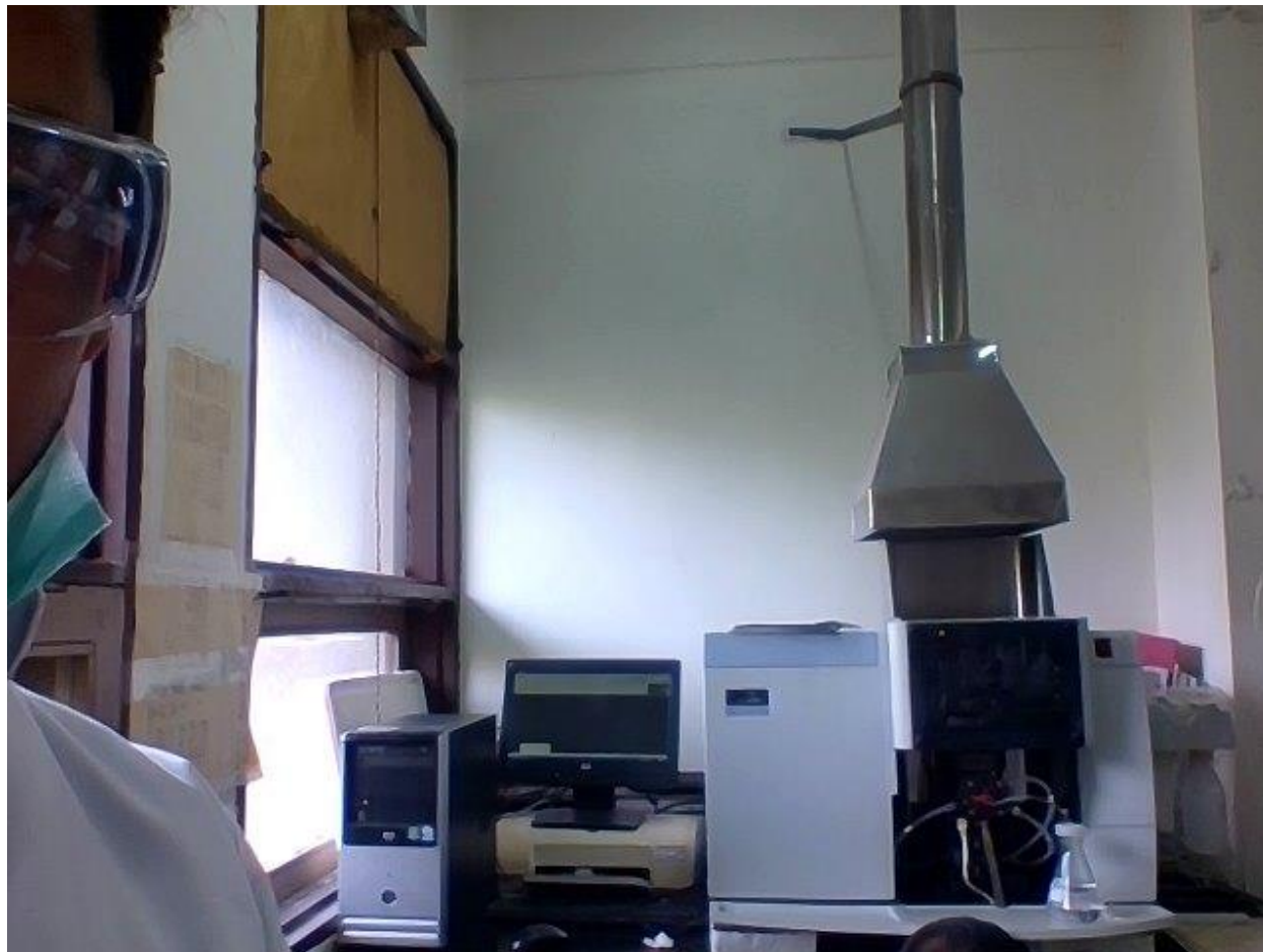
Fig No. 20 Heavy metal testing using Atomic absorption spectroscopy (PERKIN ELMER , AAnalyst 400)
