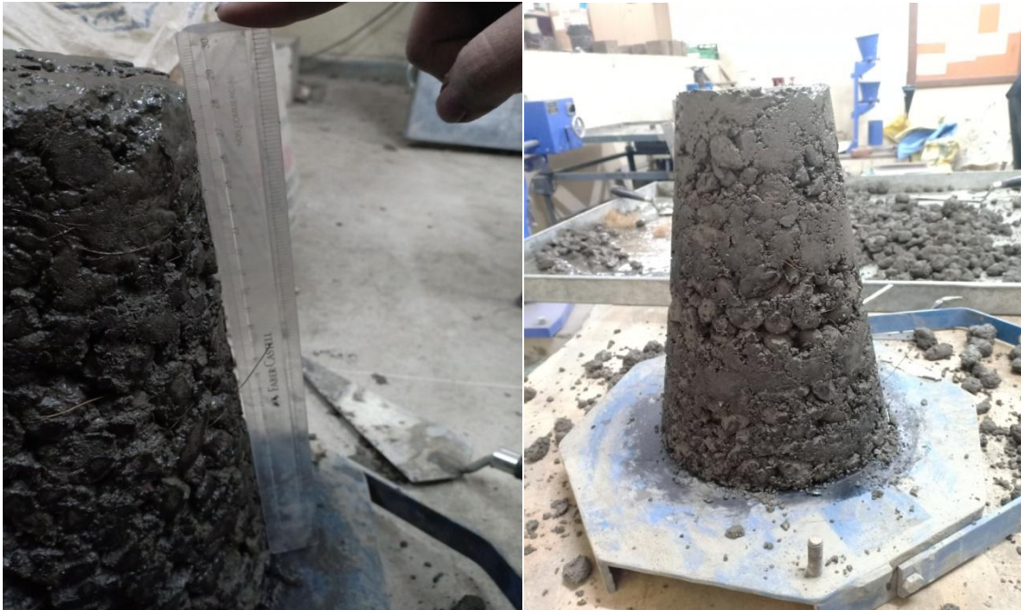
Figure 19: Workability using slump cone test.
