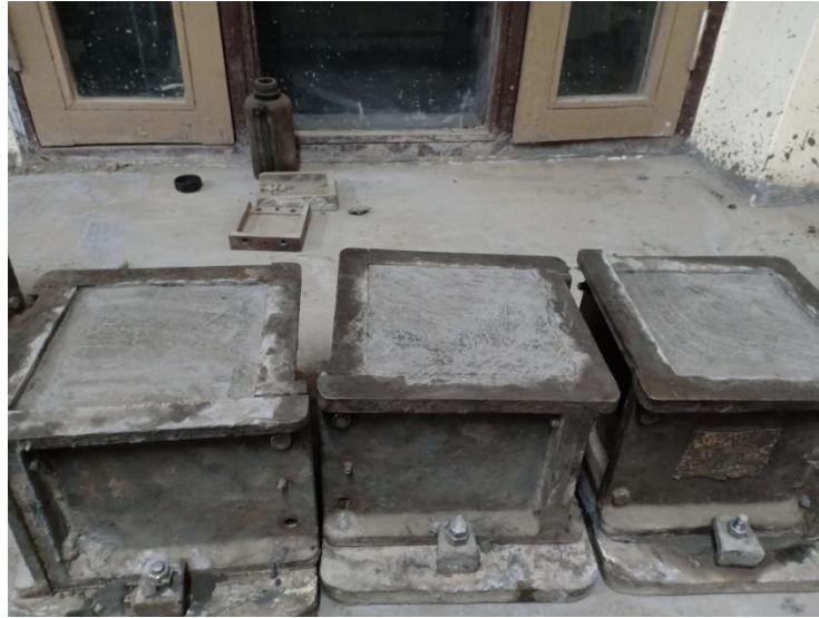
Figure 12: Casting Of Cube in Moulds
