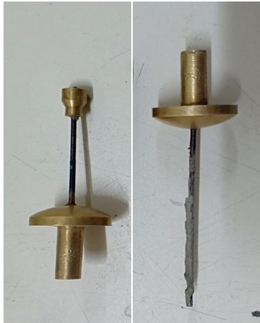
Figure 9: Needles for Initial setting time and Final setting time for cement.
