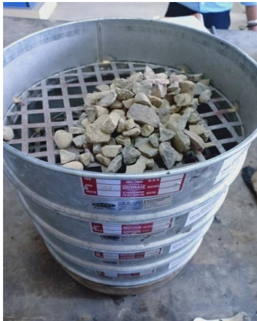
Figure 10. Sieve analysis of coarse aggregate
