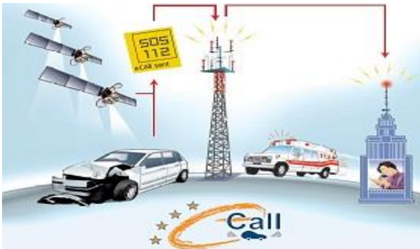
Fig 1.2.2 SOS calls system in cars.
