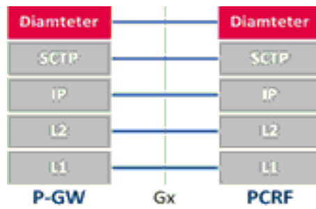
Figure 3.21 : protocol stack of Gx interface
