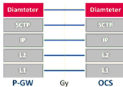
Figure 3.22 : protocol stack of Gy interface
