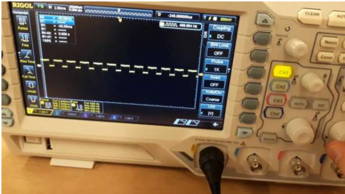
Figure 3.4 PWM output on an oscilloscope
