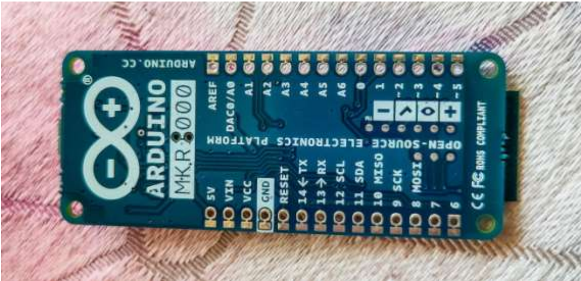
Figure 2.6: Arduino MKR1000 Pin Description (Back)
