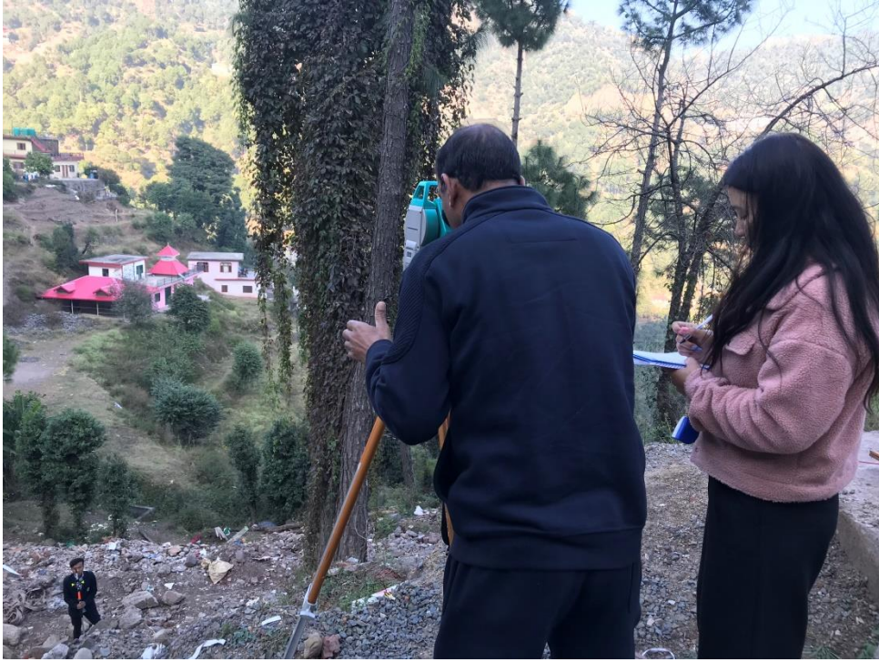
Fig3.9: Measurement of the slope using Total station
