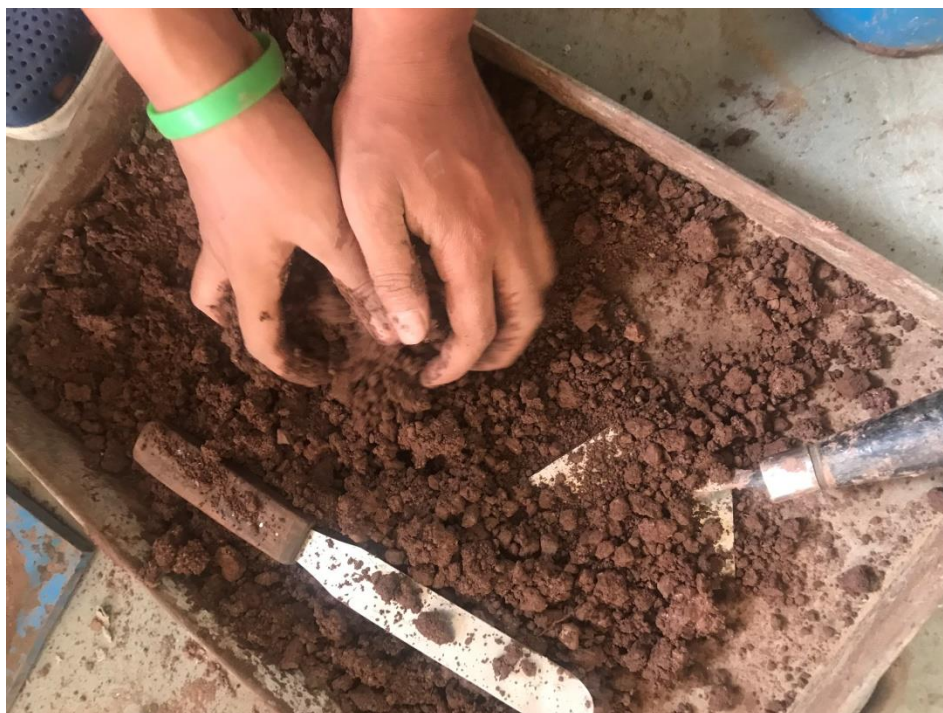
Fig3.4: Mixing of soil for the compaction
