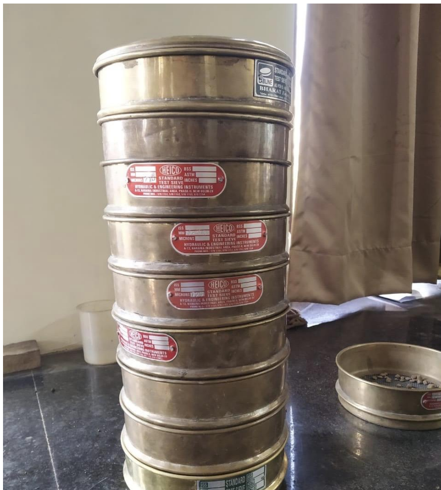
Fig3.2: Performing sieve analysis
