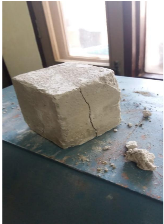
Fig 3.11 Cracking Pattern of Cub
