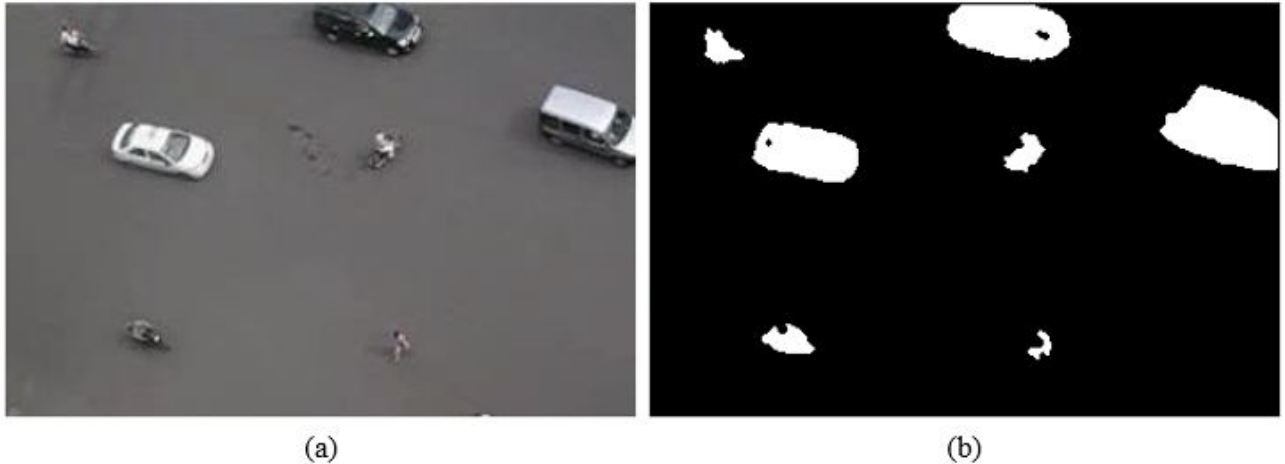
Figure 2.1: Example of vehicle detection (a) Original image (b) Detected vehicle regions
