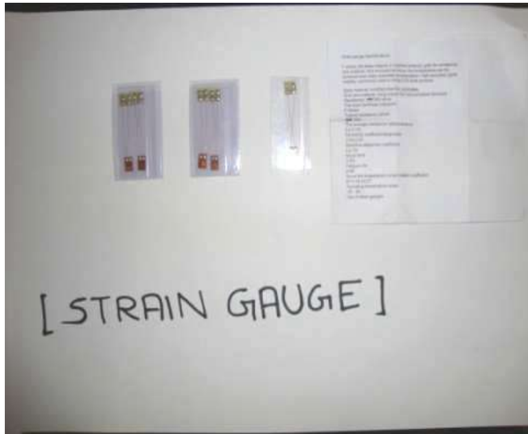
Figure 3.16 Foil type strain gauges available from National instruments, Jaipur.
