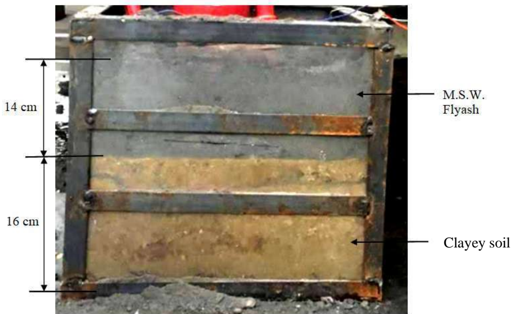
Figure 3.2 Lower layer of 16 cm clayey soil and 14 cm of M.S.W. fly ash
