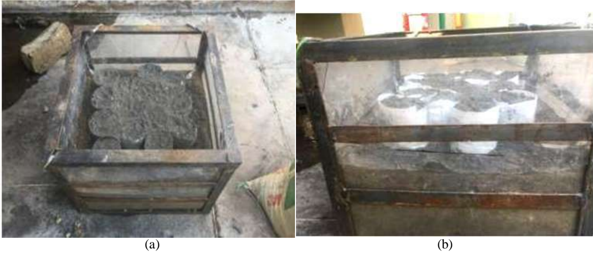
Figure 3.11 Octahedral packing shaped geocells of diameter 7cm made of polyethylene terephthalate (a) polypropylene (b) filled with fly ash are placed over the low graded clay at different heights from base of MSW fly ash or top of clayey soil
