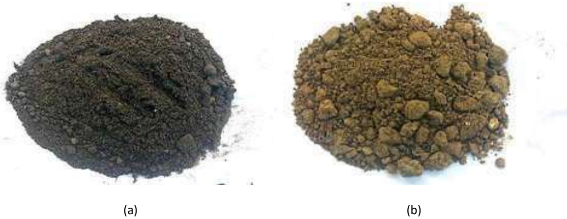
Figure 3.8 M.S.W. Flyash (left) black in colour generated from municipal solid waste incinerator Chandigarh. Organic clayey soil (right) of brown colour obtained from Armsdale building site, Shimla
