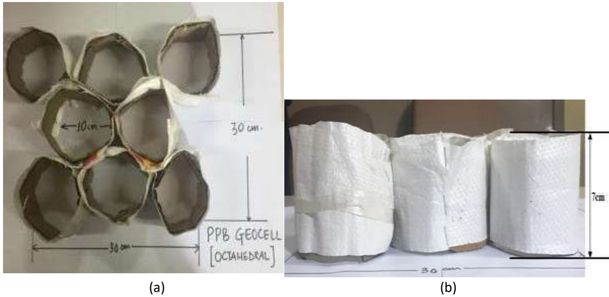
Figure 3.7 Plan (a) and elevation(b) of polypropylene bag geocells of diameter=10 cm made in octahedral arrangement
