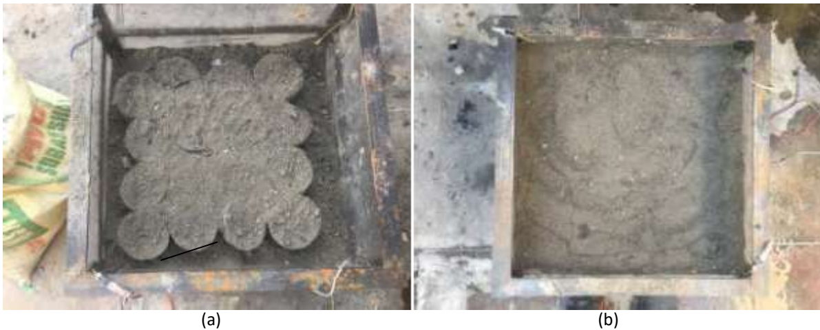
Figure 3.12 Tetrahedral packing shaped geocells of diameter 7cm made of polyethylene terephthalate (a) filled with fly ash are placed over the low graded clay at different heights from base of MSW fly ash or top of clayey soil. (b) depicts the top layer after the geocells are embedded within the entire depth of MSW fly ash ie.,14cm
