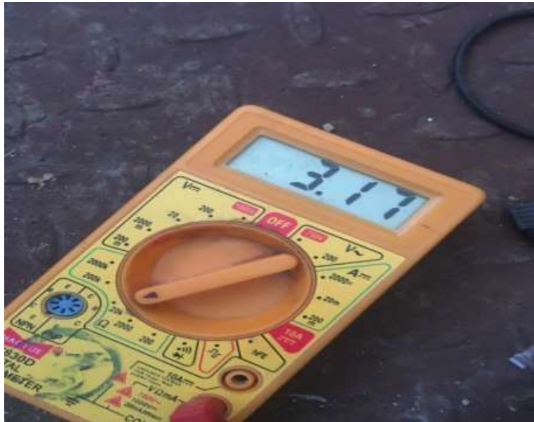
Figure 3.18 Digital Multimeter displaying initial resistance of undisturbed strain gauge in ohms.
