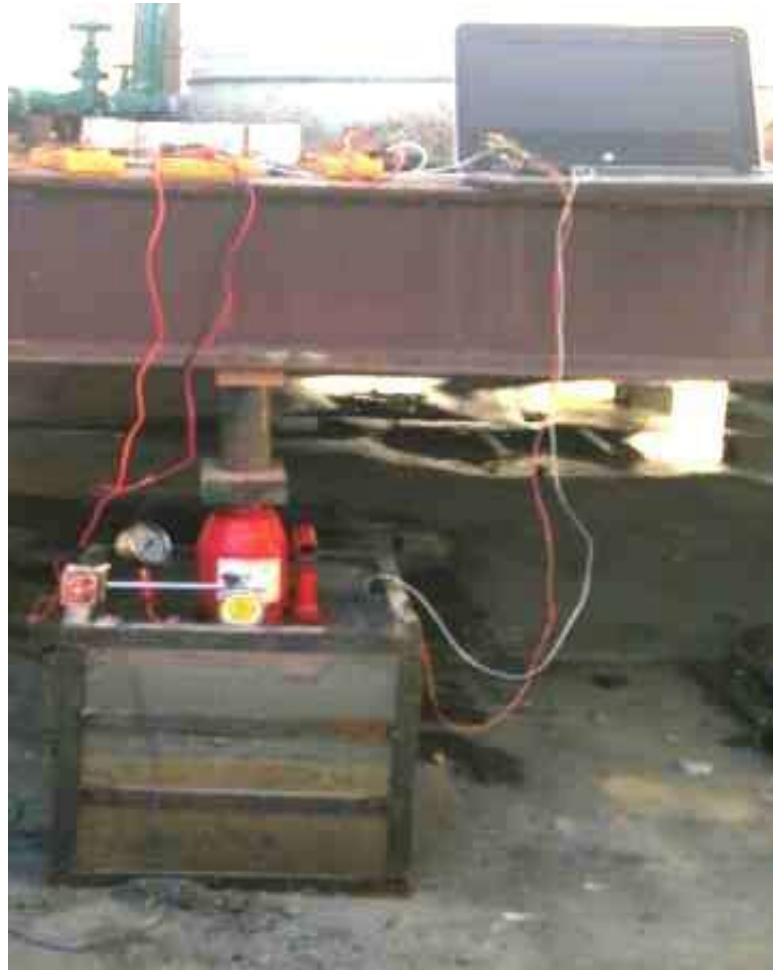
Figure 3.21 Final arrangement for model testing of various geocells
