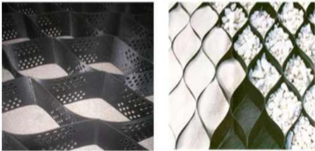
Fig. 2.4 Close view of geocells
