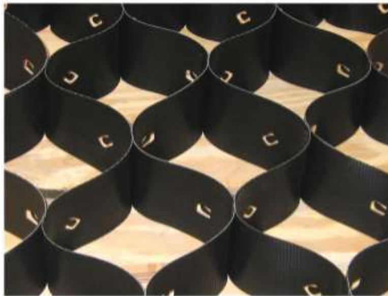
Fig. 1.5 Novel Polymer Geocells are spreaded widely over the ground and infill material is compacted using vibratory rollers. Vibratory rollers of weight 8 to 10 tonnes are allowed over the pavement. Pneumatic rollers is applied over the geocell reinforced pavement after the installation of geocells. [2]
