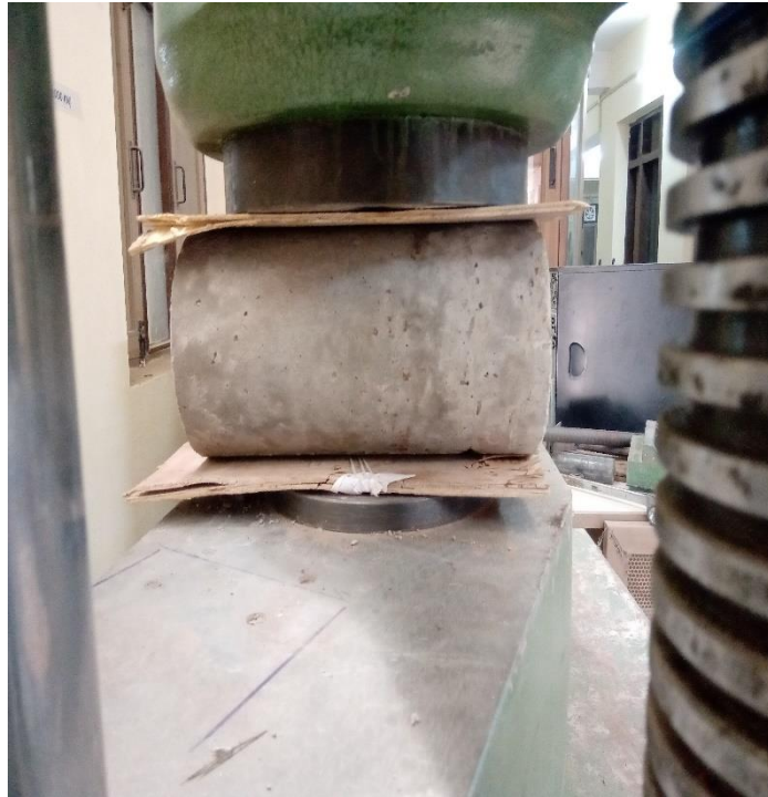
Figure 3.30 Split tensile strength test
