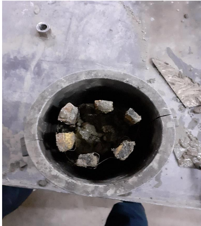
Figure 3.19 Araldite coated Reinforcement
