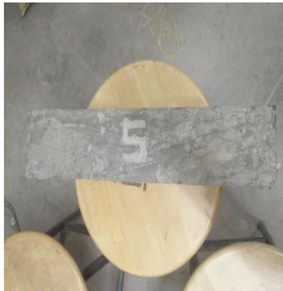
Figure 3.15 (b) BRC Beam
