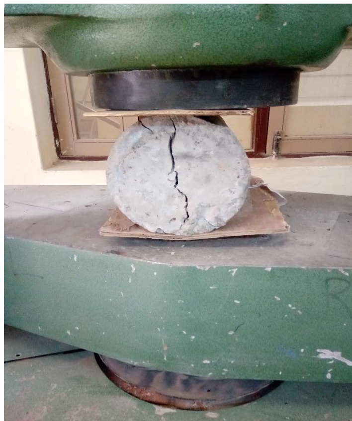
Figure 3.31 Failure of Araldite BRC cylinder
