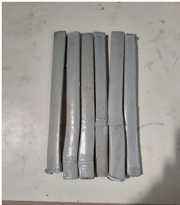
Figure 3.14 Sikadur 32-Gel Coated Bamboo Splits
