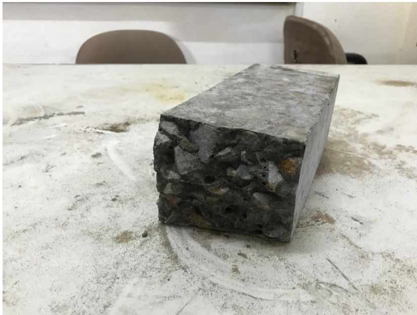
Figure 3.26 Failure of Plain concrete beam
