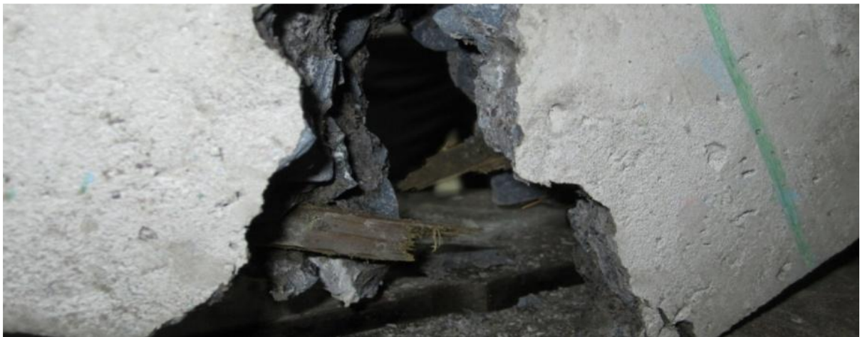
Figure 3.28 Failure of Araldite BRC beam in flexural testing
