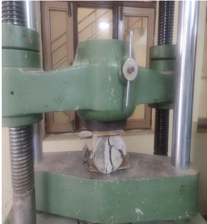
Figure 3.32 Failure of Sikadur 32-Gel BRC cylinder
