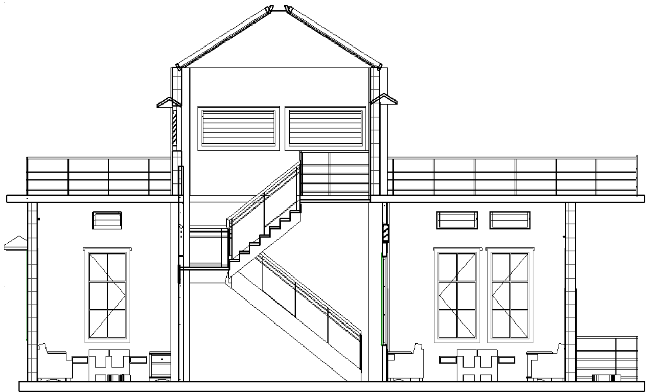
Fig.4.23 Sectional View of Stair Case Green Building
