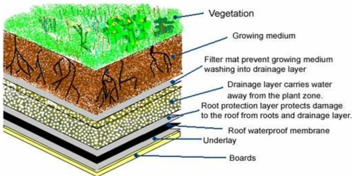
Fig.2.4 Component of Green Roof
