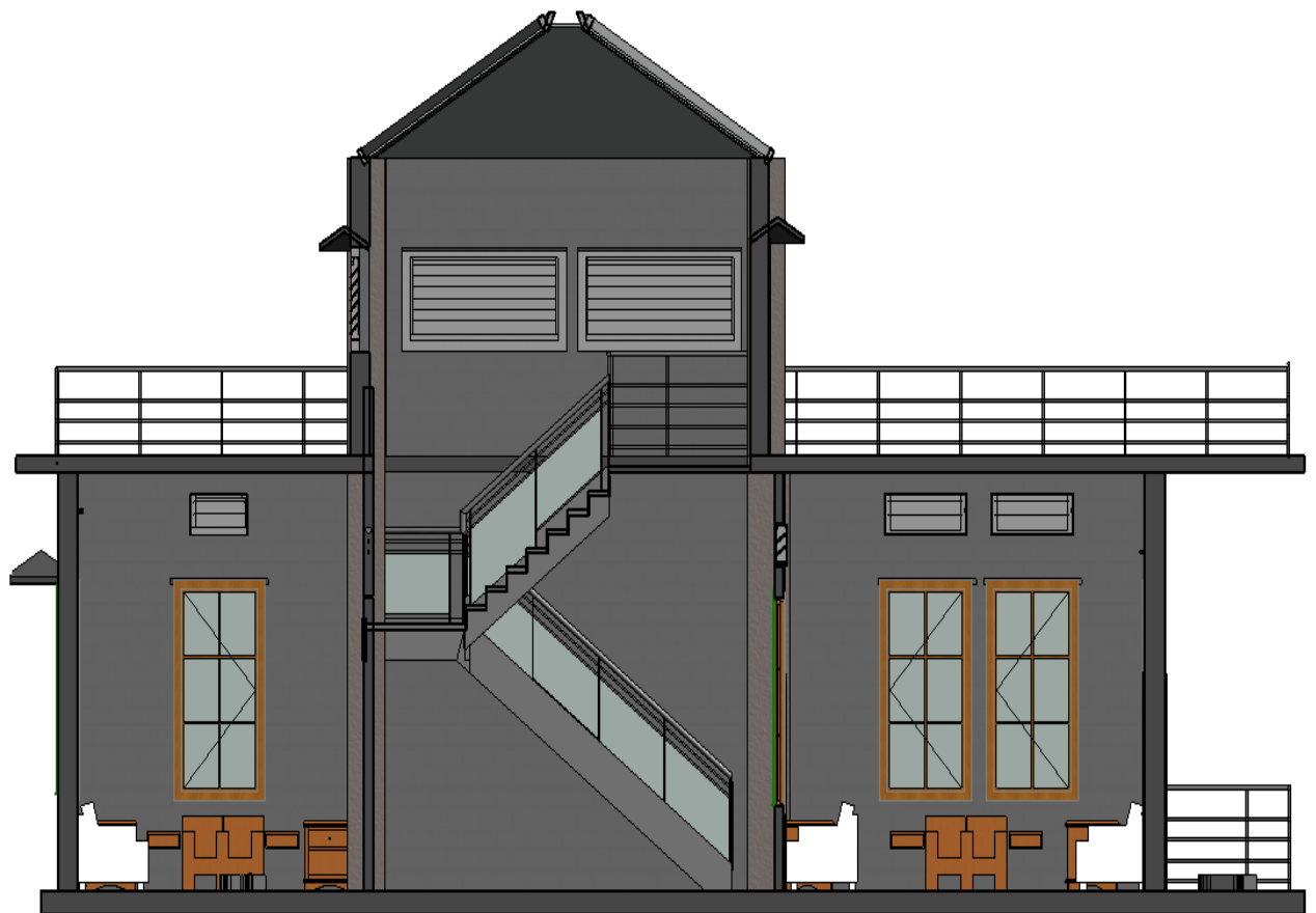
Fig.4.23 Sectional View of Stair Case Green Building
