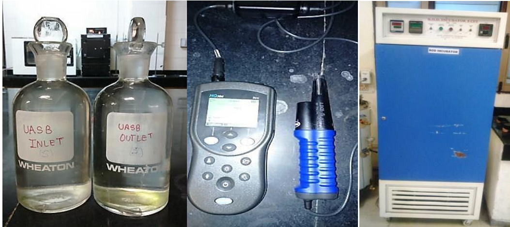
Figure 3.4: BOD Bottles Figure 3.5: Digital DO meter Figure 3.6: Incubator
