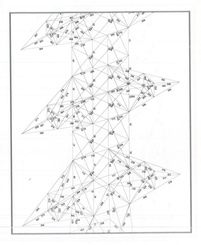
Figure-2: Portion of the Tower showing member numbers between top 7.5 m and 15 m.
