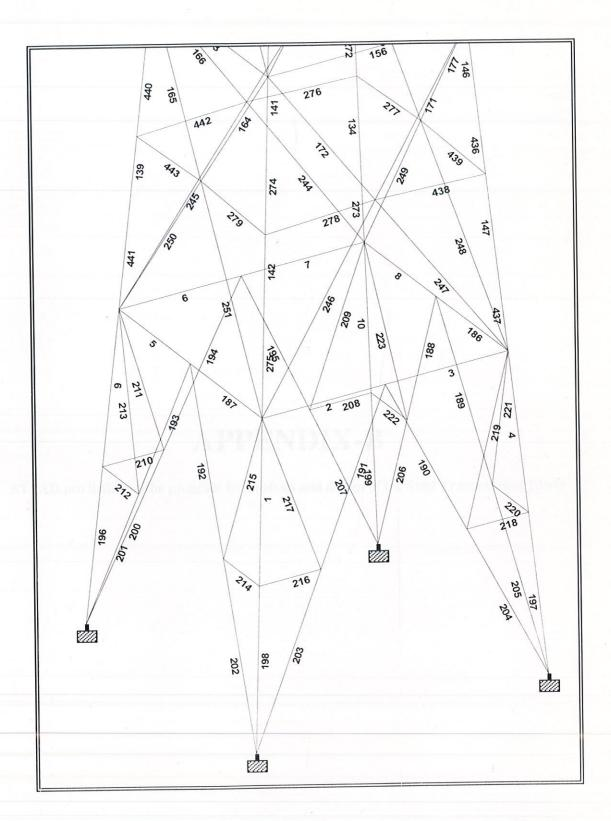
Figure-4: Bottom 10m portion of the Tower showing member numbers.
