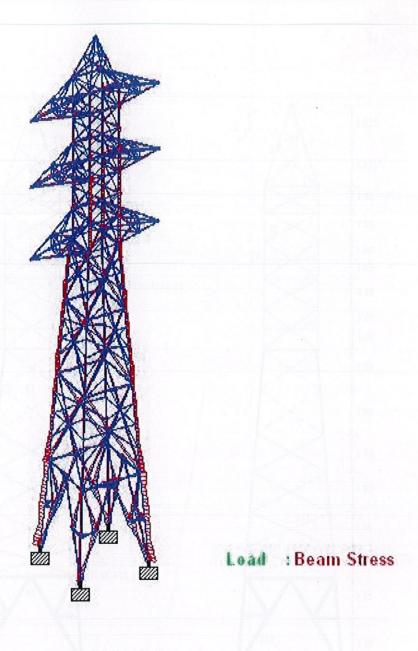
Fig. 2.4: Isometric View of Steel Transmission Tower showing stresses
