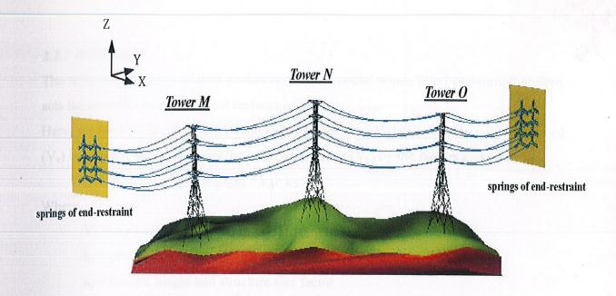
Fig. 2.6 Analytical model of tower system
