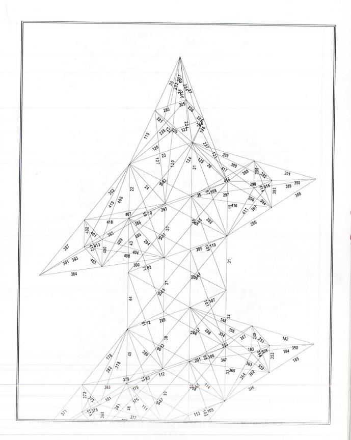
Figure-1: Top 7.5 m of the Tower showing member numbers
