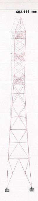
**Fig. 3.2** Displacement of the tower under Worst load combination i.e.  $[1.2 \times DL + 1.2 \times LL + 1.2 \times WL]$  in Z dir.
