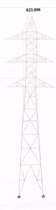
**Fig. 3.1** Displacement of the tower under Worst load combination i.e.  $[1.2 \times DL + 1.2 \times LL + 1.2 \times WL]$  in X dir.
