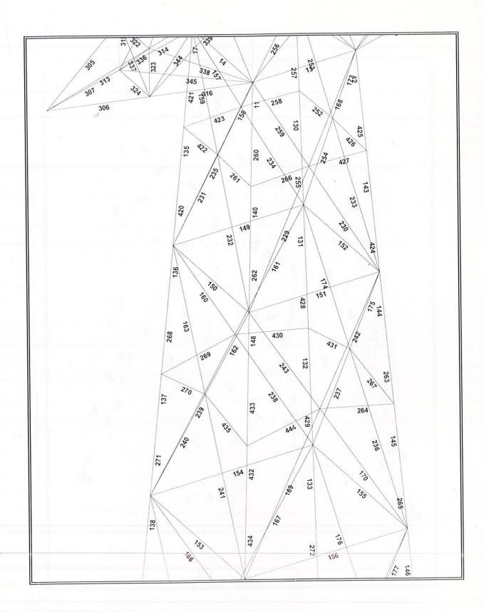
Figure-3: Portion of the Tower between bottom 10 m and 15 m showing member numbers
