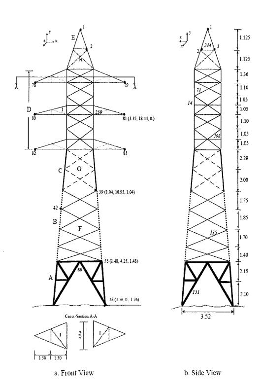
Fig. 2.5 Front view and side view of Transmission Tower
