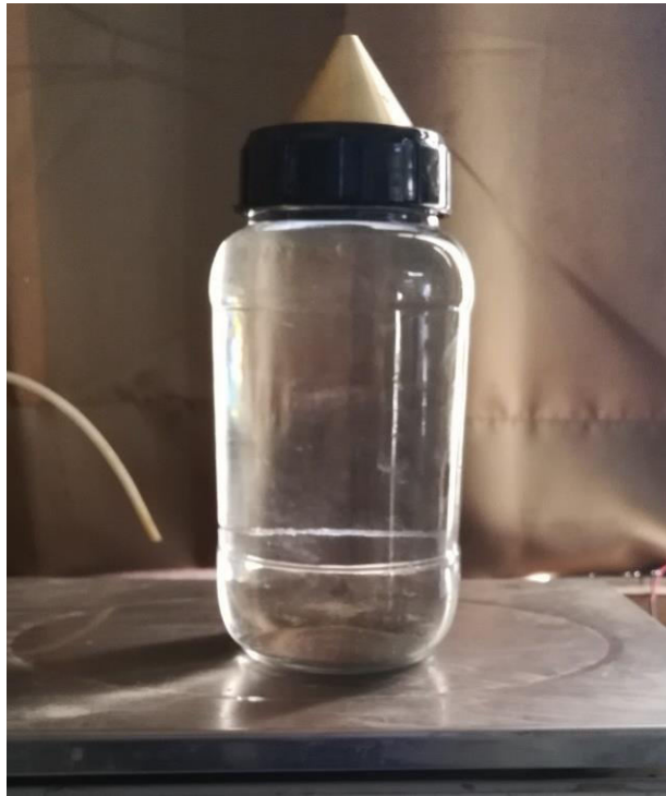
Figure 9: Pycnometer sample for specific gravity.
