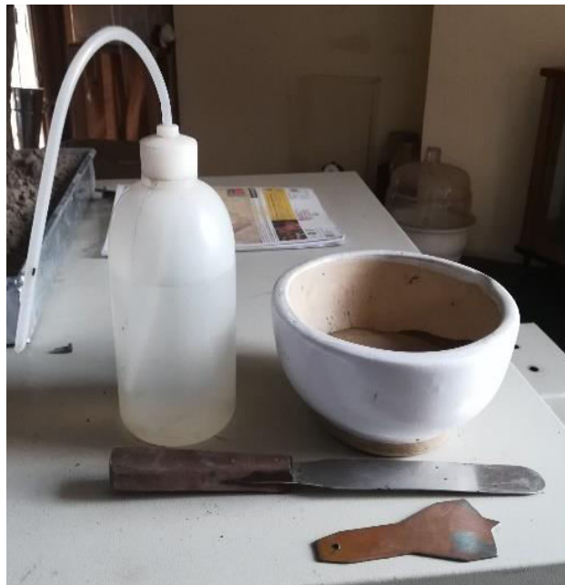
Figure: 4 Liquid limit sample.
