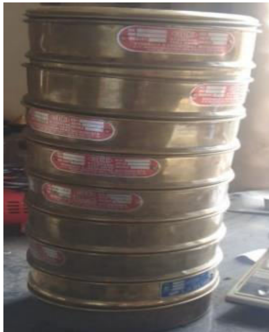
Figure 3: Sieve set for dry sieve analysis.
