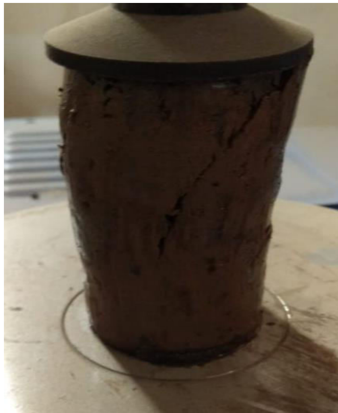
Figure 8: Sample failure of UCS.
