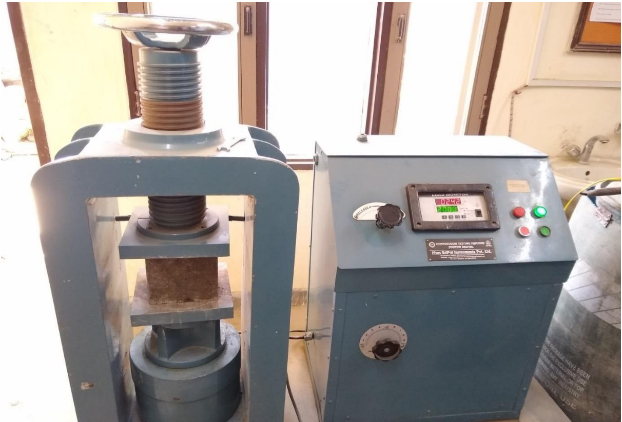
Figure 8 Compressive Strength of Concrete
