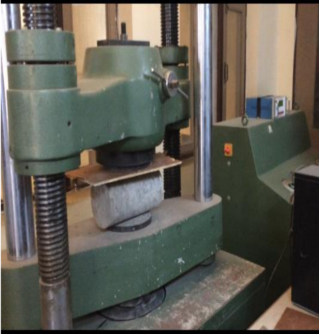
Fig.10 Finding Split Tensile Strength
