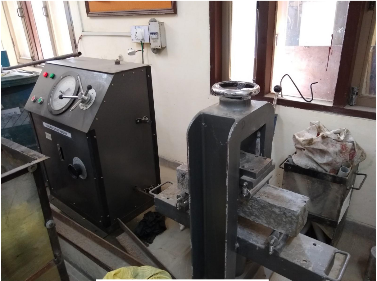
Fig.9 Finding Flexural Strength
