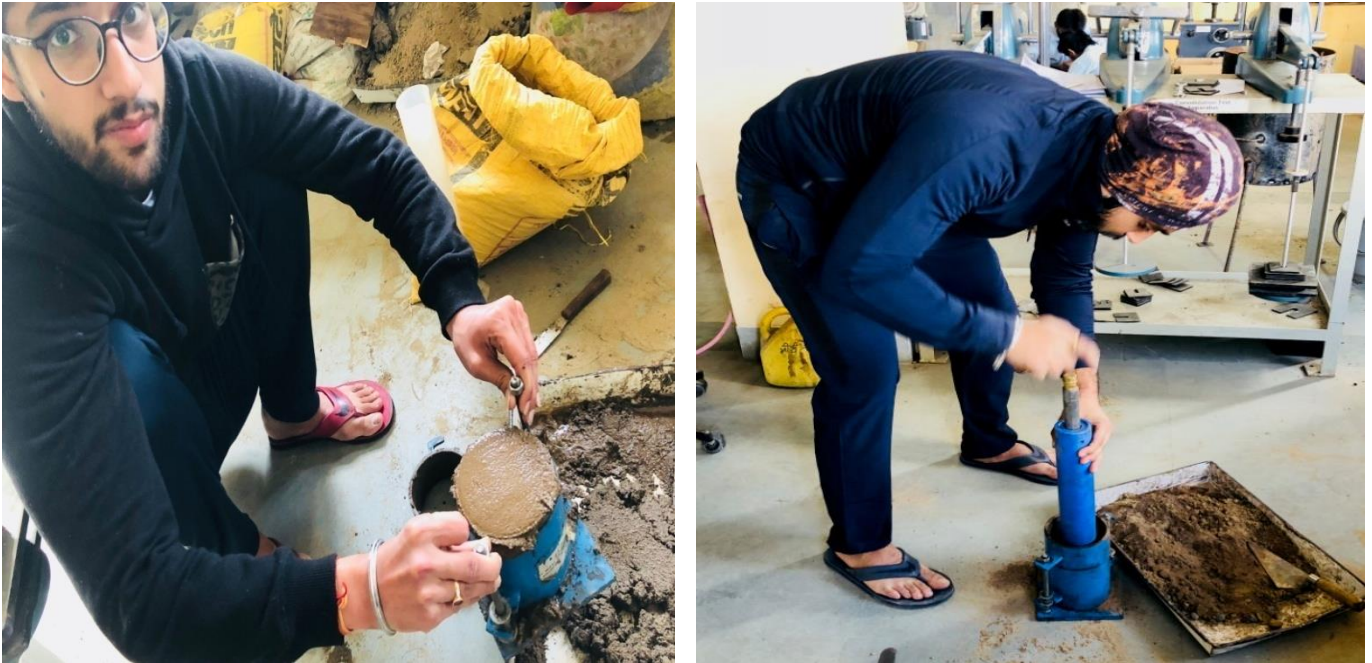
Fig. 3. Performing Standard Proctor Test in Laboratory
