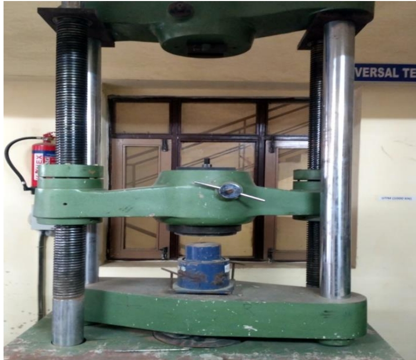
Fig 3.7 Crushing value setup
