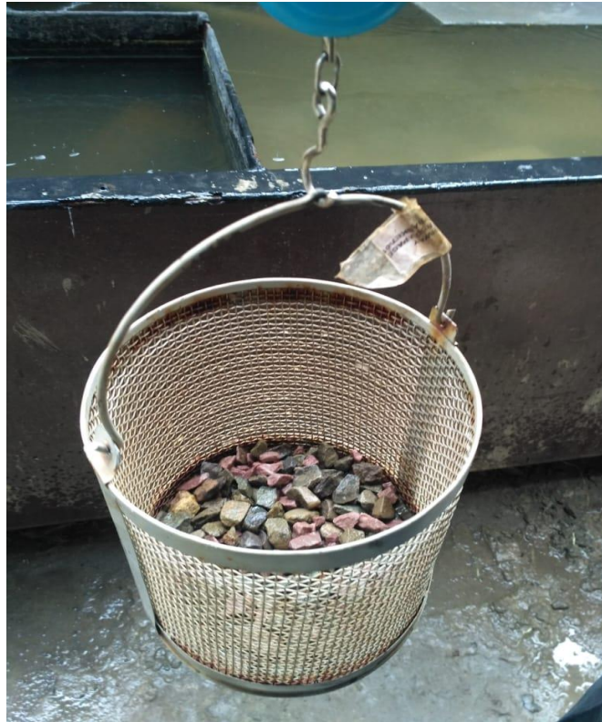
Fig 3.8 Water Absorption test
