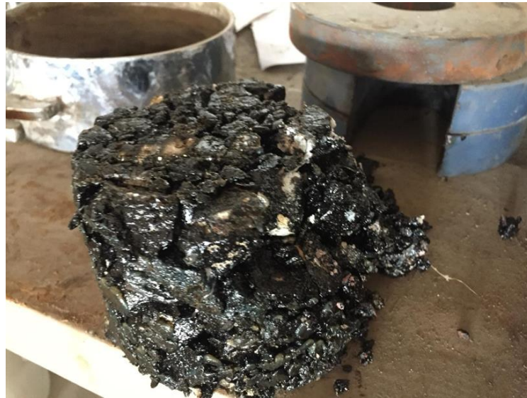
Fig 4.6 Sample failed at 3% replacement of Waste engine oil
