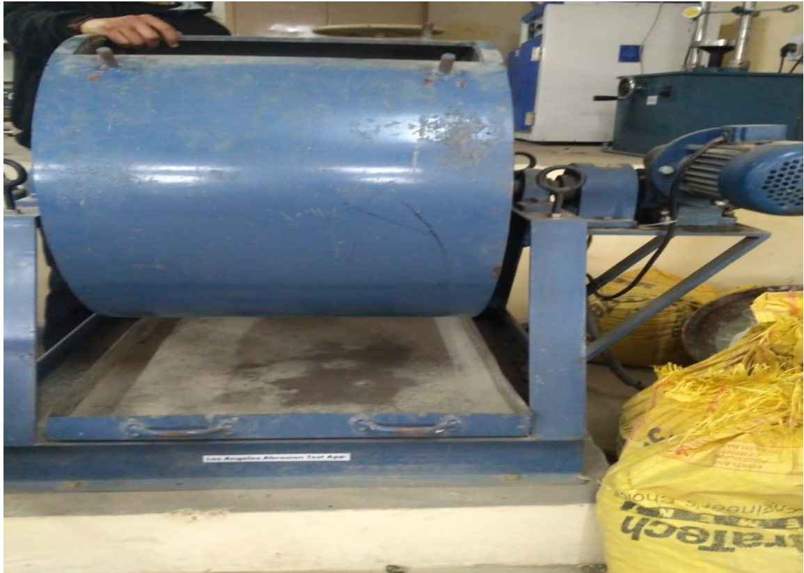
Fig 3.10 Los-Angeles test setup
