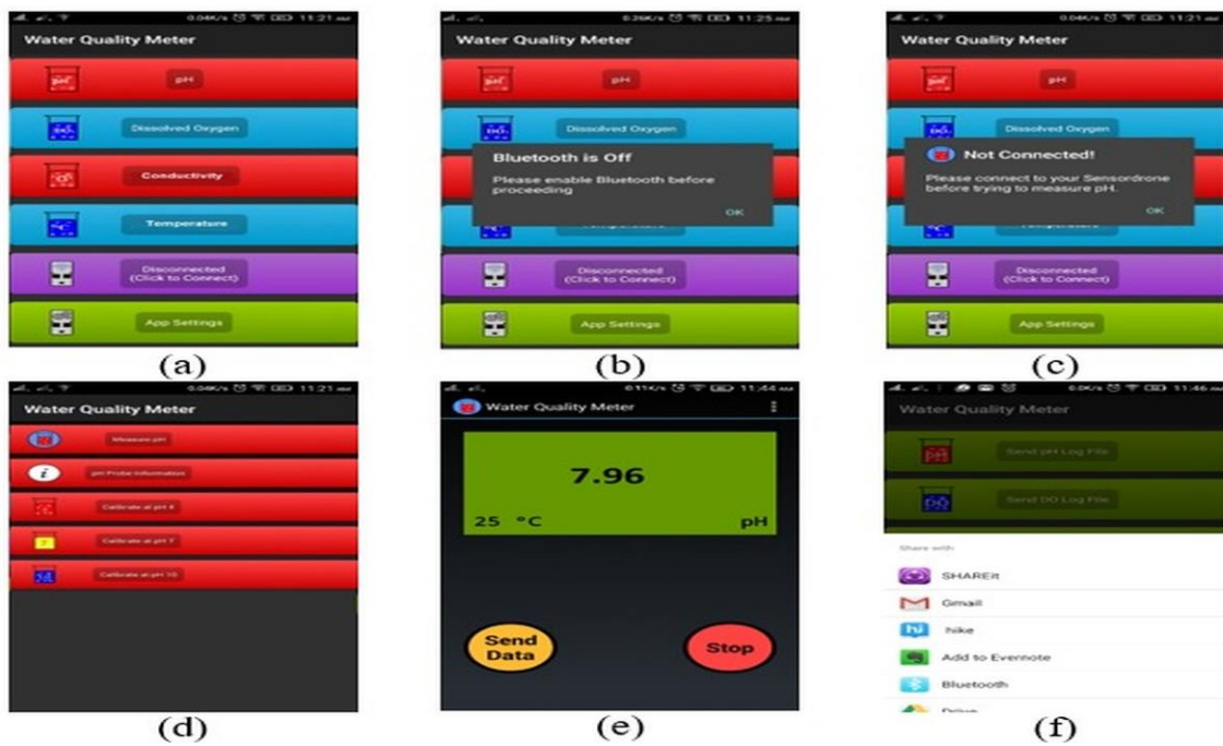
Figure 3.3: Data collection using smart-phone software (a) home screen, (b) prompts for enabling Bluetooth, (c) checking nearby devices, (d) data gathering, (e) data processing and (f) data sharing with external applications
