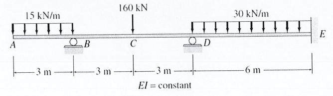
Q.3 Find the deflection of joint 'C' along y axis of the frame by using unit load method. Assuming EI is constant for the frame. (6)
