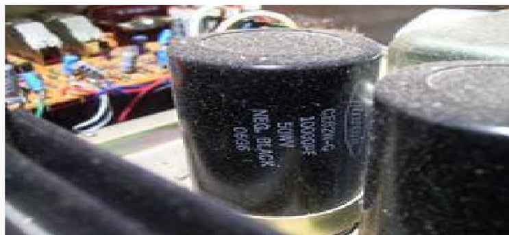
Figure 3.2 10 millifarad capacitor in an amplifier power supply
