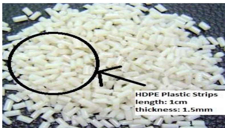
Fig.3: view of HDPE strips
