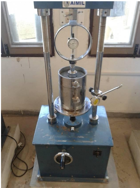
Fig 10: CBR test apparatus and sample
