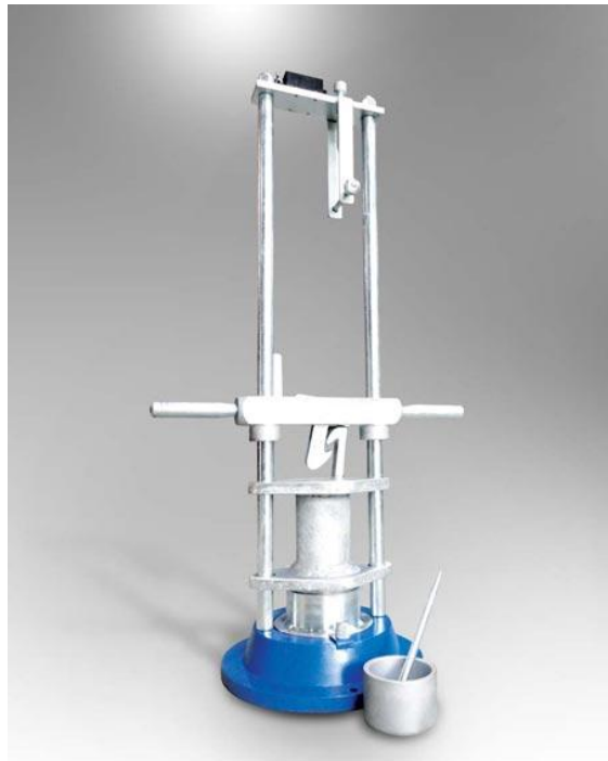
Fig 15: Impact Value Test apparatus
