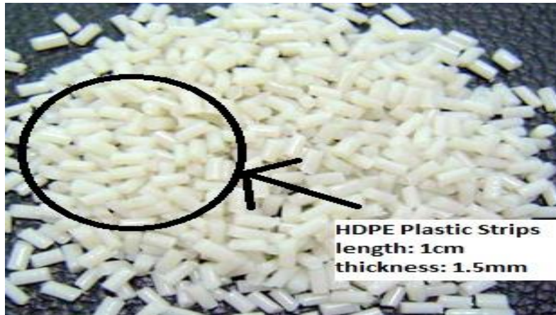
Fig.3: view of HDPE strips
