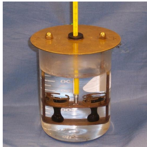
Fig 13: Ring and Ball test apparatus
