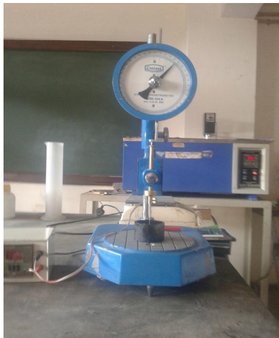
Fig 11: Penetration Test Apparatus
