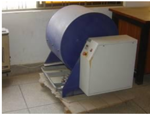
Fig 14: Los Angeles Abrasion Test apparatus
