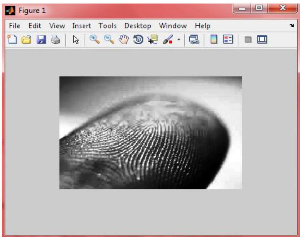
FIG 10: GABOR FILTER USED ON THE ENHANCED IMAGE.
