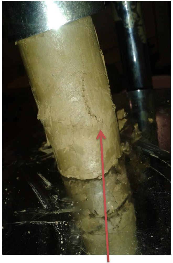
Failure with Woven Geotextile when kept uniformly spaced in between the sample
