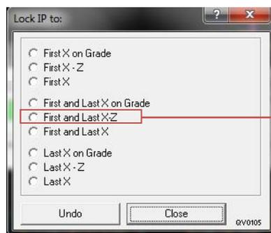
This one will lock the position of first and last IP to the starting and end of horizontal alignment
