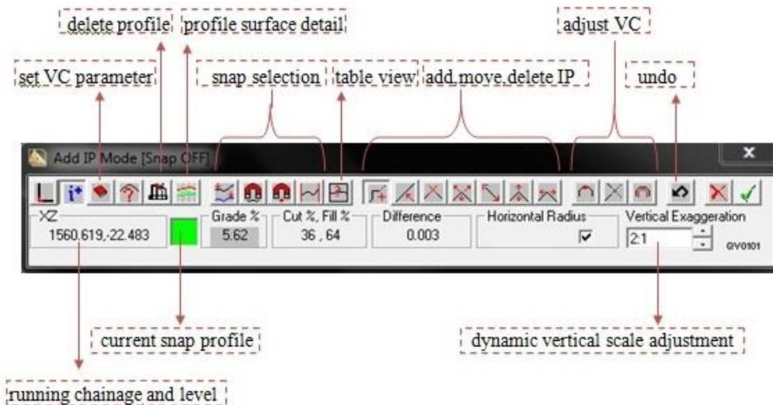
Figure A9 Quick Vertical Alignment Toolbar
