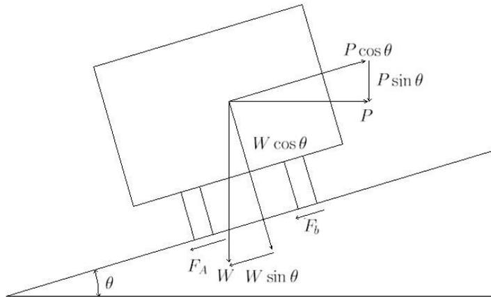
Figure 2.2. Analysis of super-elevation
