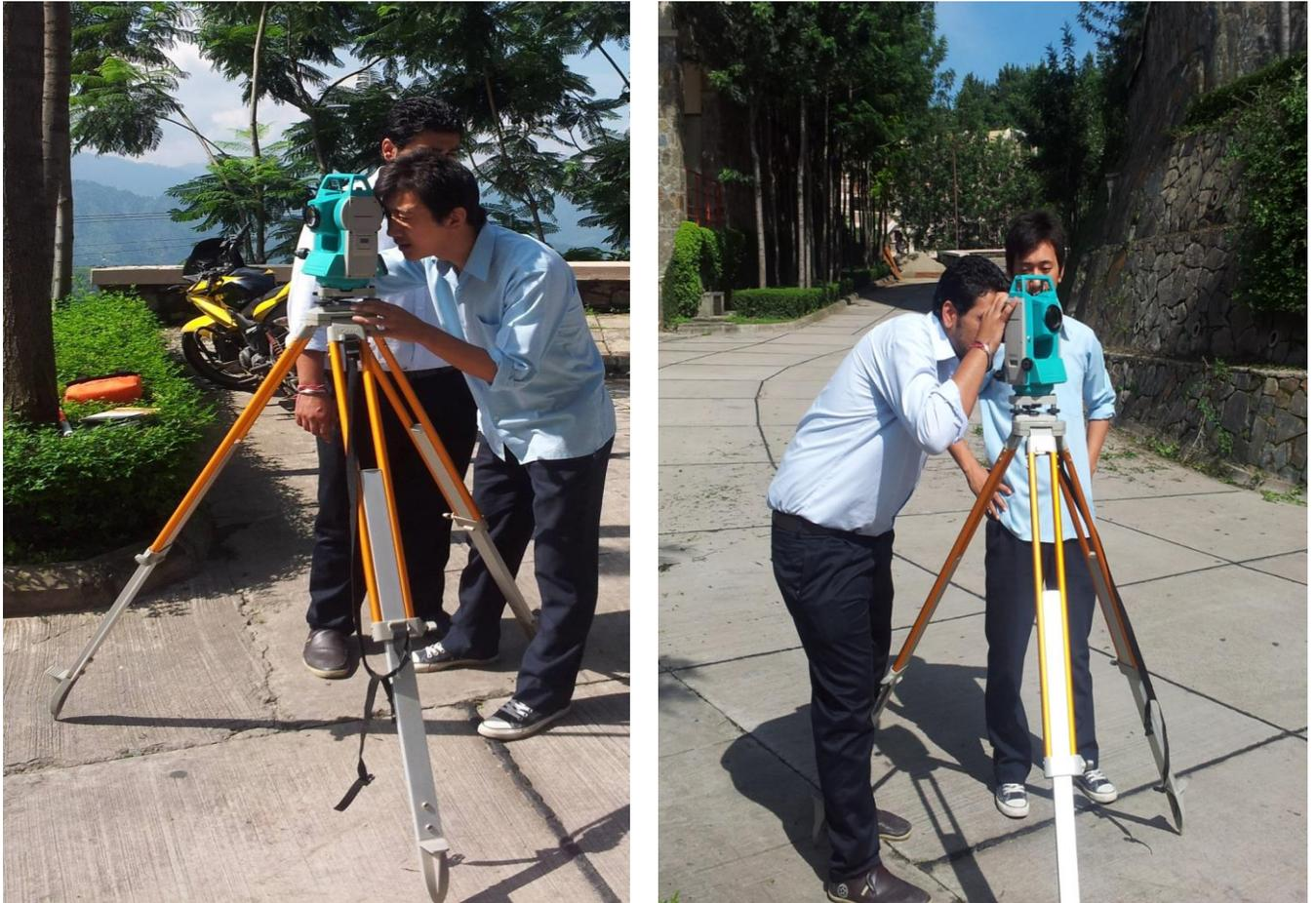
Figure 3.5 Trial survey using total station in JUIT campus, under progress
