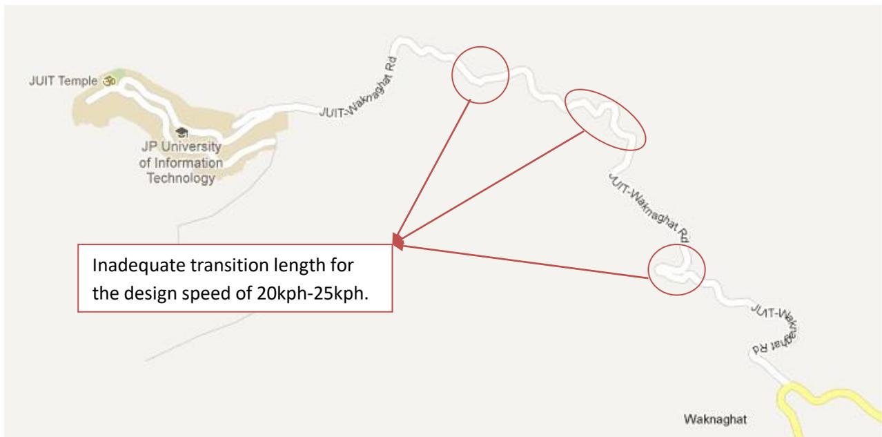
Figure 4.2 Inadequate transition length for the selected road stretch
