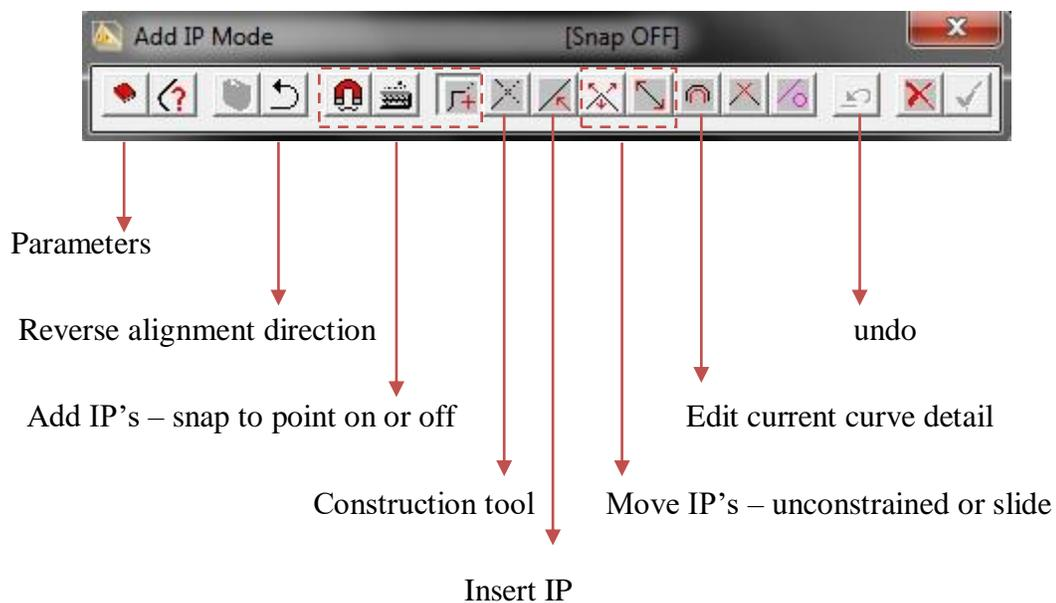
Figure A8 Quick Horizontal Alignment Toolbar
