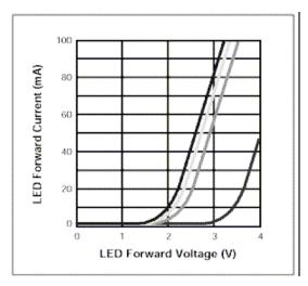
Fig. 22 Graph representing Voltage vs. Current
