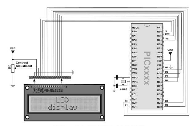
LCD HW connection by default initialization (using Lcd8\_Init)
