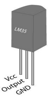
Fig.10 Temperature Sensor (LM35)
