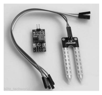
Fig.13 Soil Moisture Sensor
