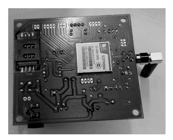
Fig.3 Bottom view of GSM modem
