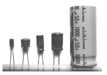
Fig 19. Electrolytic Capacitors
