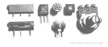
Fig 17. VARIABLE RESISTORS
