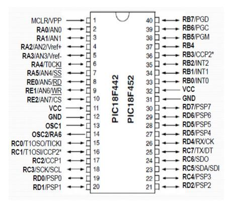
Fig.24 Pin diagram of PIC MCU
