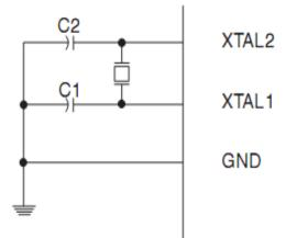
Fig.14 Connection of Crystal Oscillator with PIC MCU
