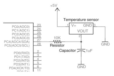
Fig.11 Connection of LM35 with PIC MCU
