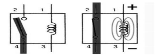
Fig.9 Internal view of Relay
