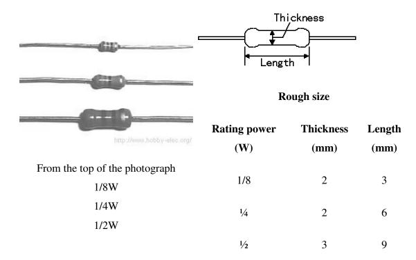
Fig.16 Physical size of the different resistors
