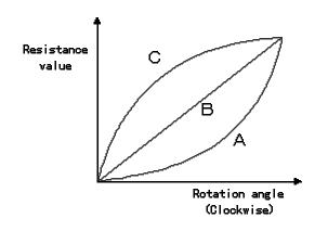
Fig 18. Resistance value vs. Rotation angle
