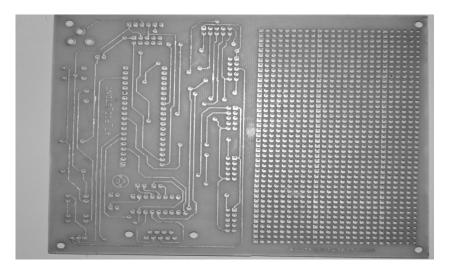
Fig.15 PCB for PIC MCU
