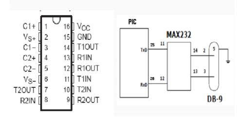
Fig.5 Pin diagram of MAX 232
