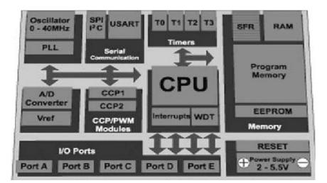
Fig. 1 Architecture of PIC MCU
