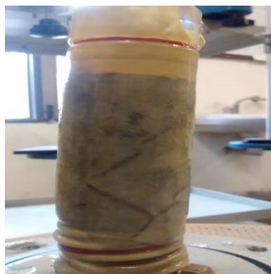
FIG.6 FAILED SAMPLE IN CU TEST
