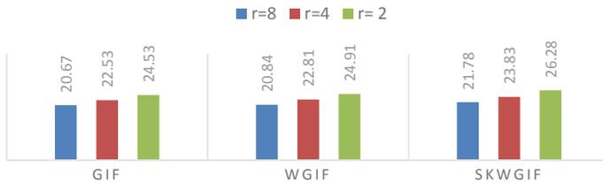
Fig. 2 PSNR values of different guided filters [7]
