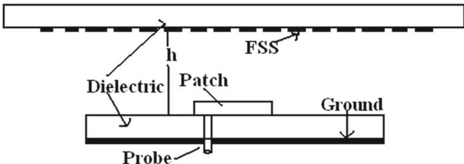
Fig. 3 The frequency selective surfaces superstrate antenna with the reduced ground plane size
