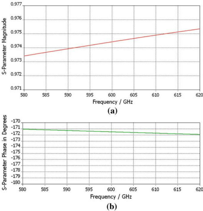
**Fig. 2** Frequency response of the frequency selective surface (a) magnitude and (b) phase angle
