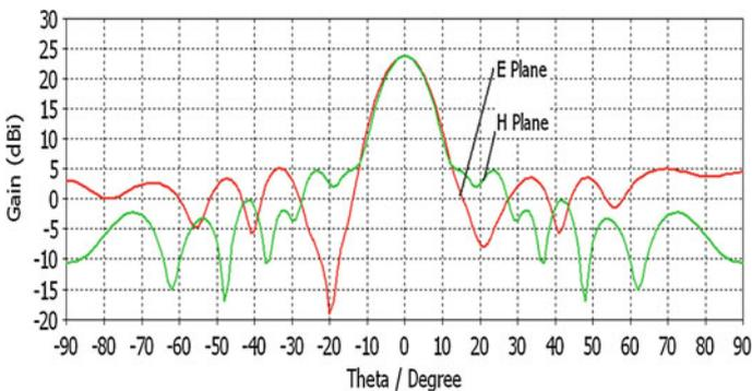
**Fig. 11** Gain of the scaled down antenna at 297 GHz
