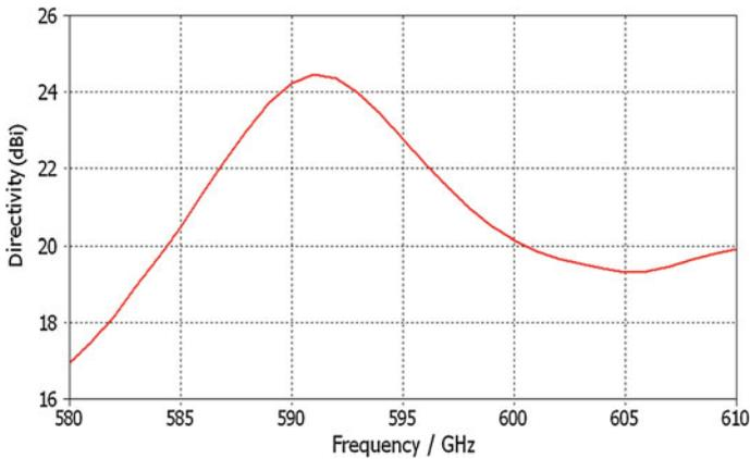
**Fig. 10** Directivity pattern of the proposed antenna over a wide frequency range
