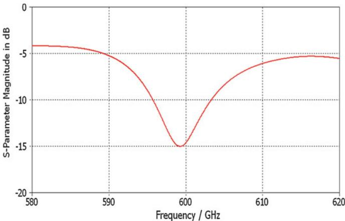
**Fig. 7**  $S_{11}$  (dB) parameter of the antenna proposed in Fig. 3
