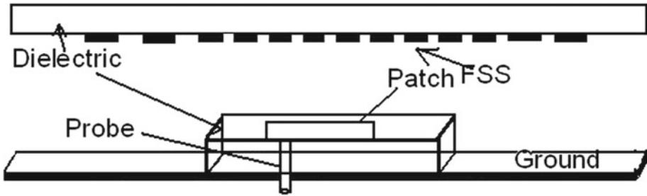
**Fig. 4** The frequency selective surfaces superstrate antenna with the extended ground plane size
