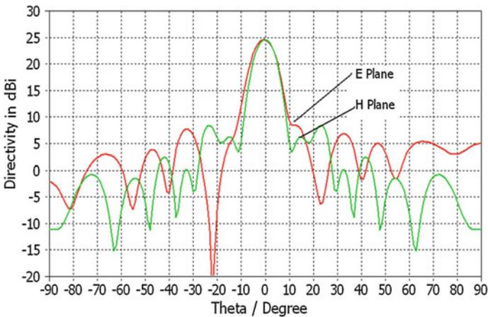
**Fig. 9** Radiation pattern of the antenna at 592 GHz
