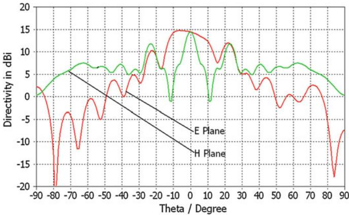
**Fig. 6** Radiation pattern of the antenna shown in Fig. 3 at 600GHz
