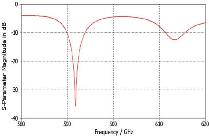
**Fig. 8**  $S_{11}$  (dB) parameter of the proposed antenna in Fig. 4
